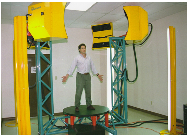
Fig. 6.1 Early Cyberware scanner with a rotating platform (from Flickr user NIOSH).
