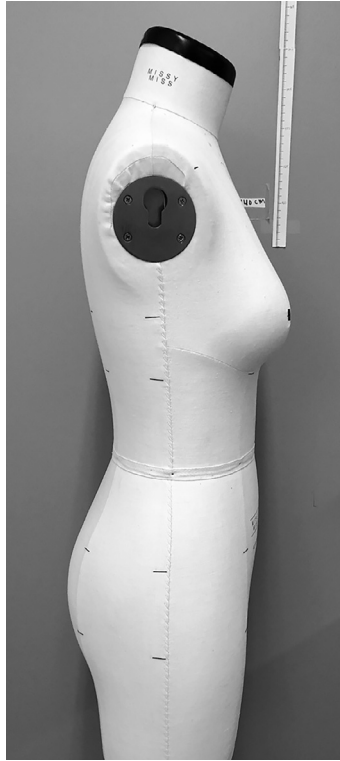
Fig. 6.6 Alvanon dress form modeled from a 3-D body scan. Unlike the traditional simplified dress form shapes used in clothing design, this form provides the anatomical curve of the buttocks and the undercut below the bust.
