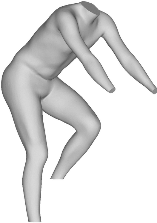
Fig. 6.13 Image of a body scan of a study participant on a bicycle. The ability to scan participants in active positions (which requires a large scan volume) allows researchers to investigate how body dimensions vary when the body is in motion.
