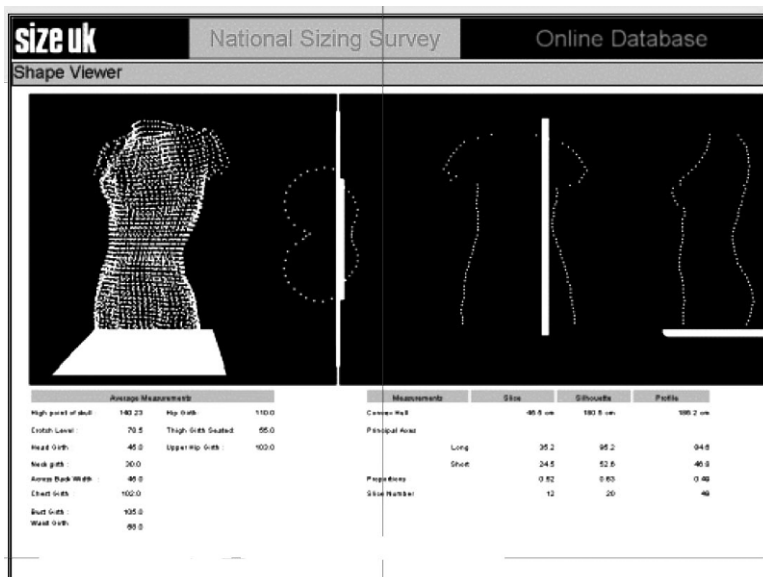
6.5 Screen shot captured in 2002 by the SizeUK team, showing web-based software tools for 3D data analysis. The online software allows the user to view (images, left to right) 3D shape analysis, seated 2D cross section, the front silhouette and side profile; and in the panel of figures below (not legible as recorded more than a decade ago) are sets of automatically generated one, and two, dimensional measurements.
