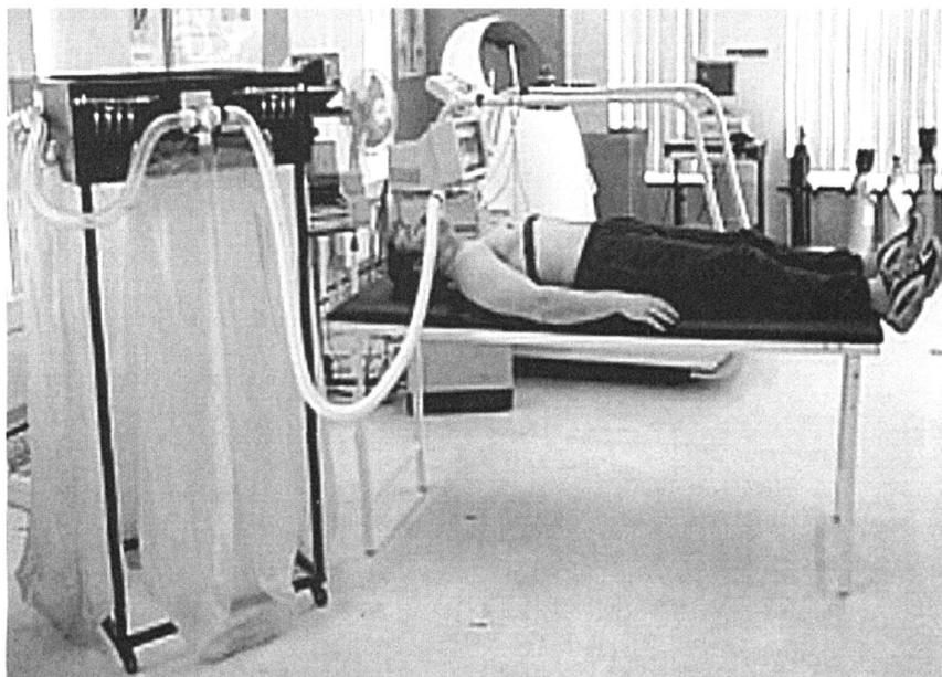
**Figure 6.1** A subject lying in a supine position in a laboratory practical for the estimation of resting metabolic rate (RMR). Expired air collection is through a mouthpiece attached to a Salford valve (Cranlea and Company, Birmingham, UK) and lightweight tubing, which is connected to a Douglas bag. The subject is wearing a nose clip, and heart rate data are being recorded by a short-range radio telemeter (Polar, Finland).
