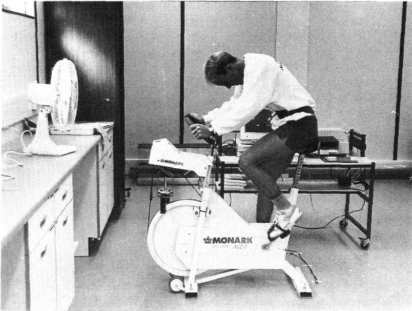
**Figure 11.1** General layout of the equipment used in the Wingate Anaerobic Test. The cycle ergometer is bolted to the floor and has a modified load hanger. Note also the use of toe clips and a restraining belt.
