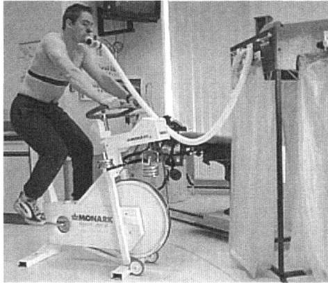
**Figure 6.2** A subject on a standard Monark cycle ergometer (Monark Crescent AB, Varberg, Sweden), with expired air collection to a Douglas bag, and heart rate monitored by a short-range radio telemeter (Polar, Finland).
