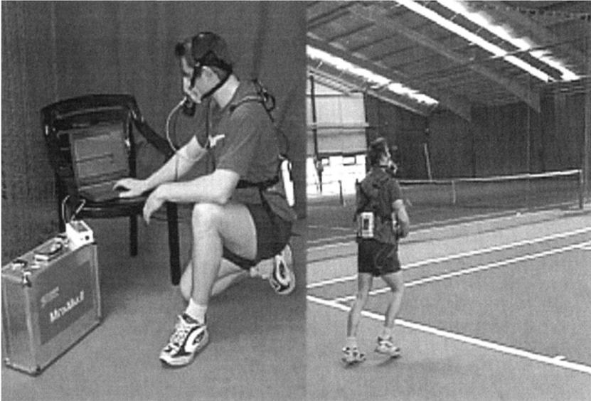
**Figure 6.4** A portable gas analysis system (MetaMax II, Cortex, Germany) to collect individual energy expenditure values for tennis. The left-hand photograph shows the system being initialised to work via telemetry, sending the signals from the device whilst the subject is playing tennis (right-hand photograph). Alternatively, the device can be used in data logging mode, with the data downloaded to the computer after the game has finished.
