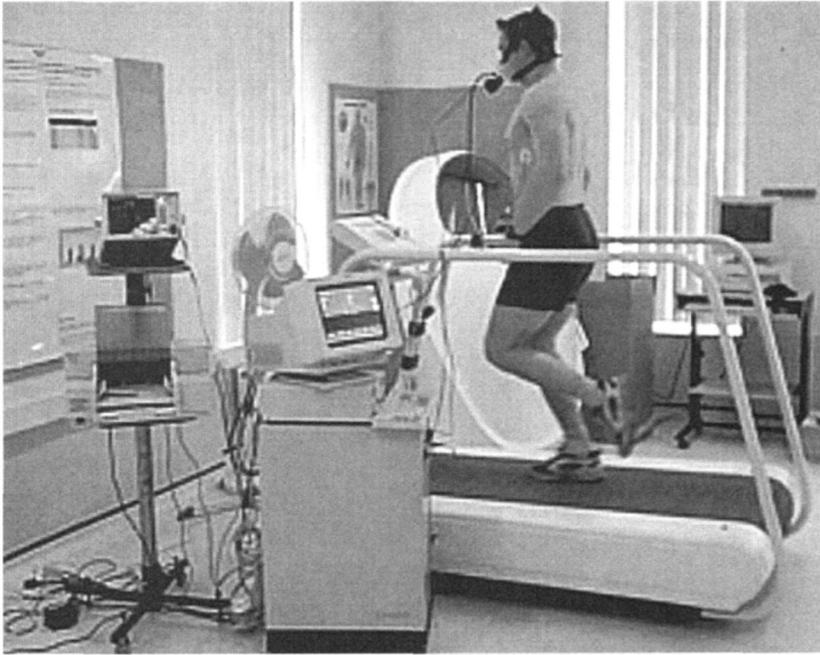
**Figure 6.3** A subject running on a motorized treadmill, with expired air analysis through a face mask (Hans Rudolph Inc., KS, USA) connected to an on-line automated breath-by-breath gas analysis system (Oxycon Champion, Mijnhardt, Bunnik, Netherlands; Jaeger, Hoechberg, Germany) and a three-lead ECG through an ECG Oscillograph (CR7 Cardiometer, Cardiac Recorders, Enfield, UK).
