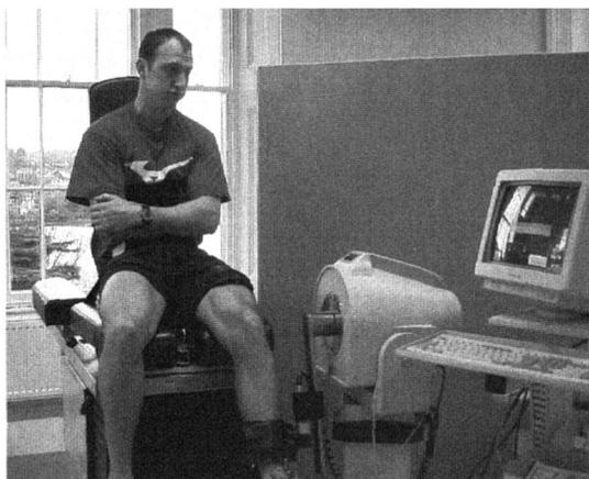
**Figure 1.5** Measurement of knee extensor strength on an isokinetic dynamometer (KinCom 500H, Chattex, Chattanooga, TN, USA).
