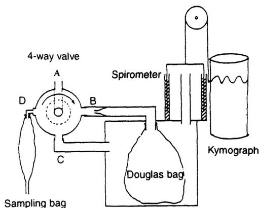
**Figure 3.11** Conventional manual system for  $DL_{COsb}$ . (Modified from Ferris, 1978.)
