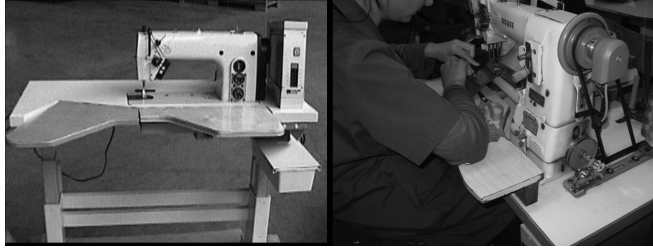
Figure 5.26 New ergonomically designed sewing tables and position of elbows at work
