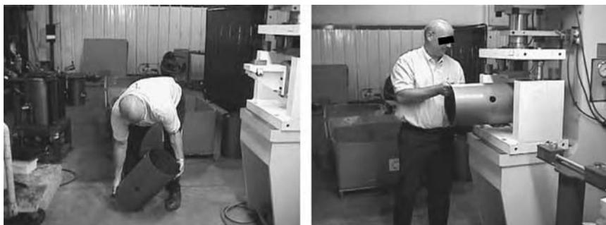
**FIGURE 50.4** Lifting shell to press.
