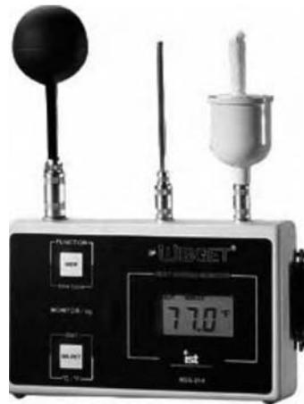
**FIGURE 62.1** Heat stress monitors.
