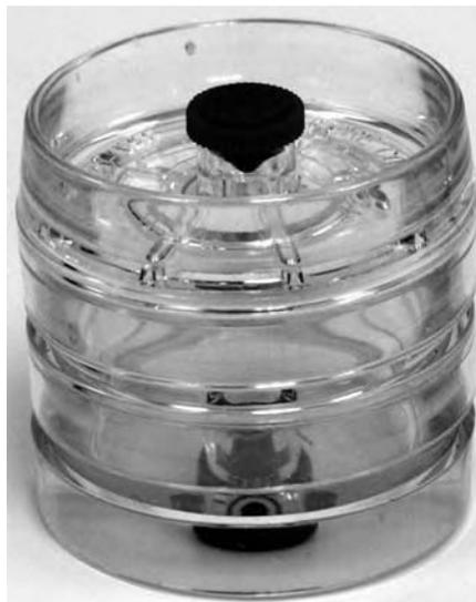
FIGURE 64.7 Filter cassette for collecting dust samples.
