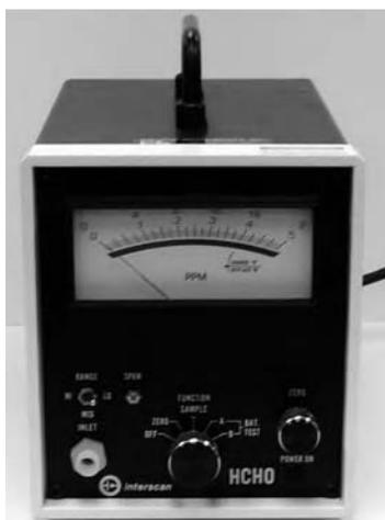
FIGURE 64.3 Direct-reading formaldehyde meter.
