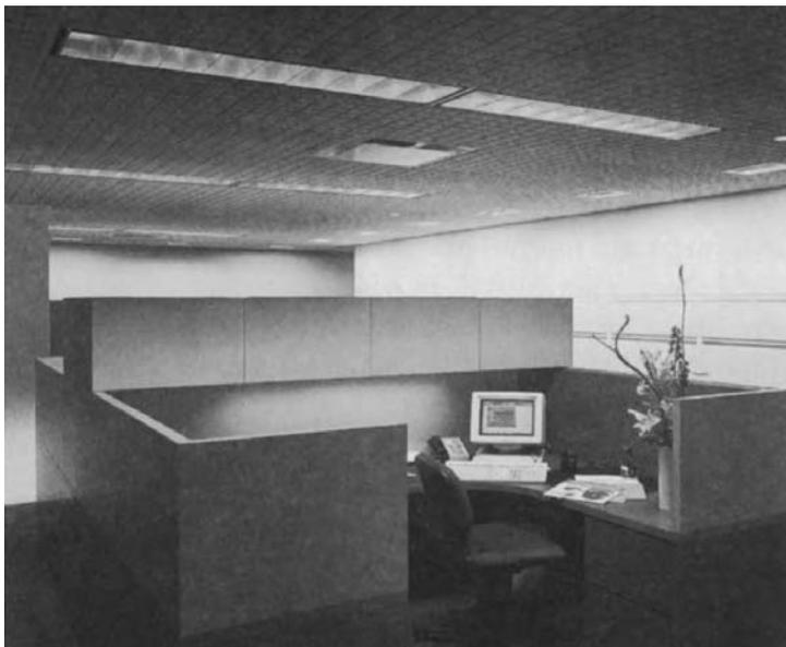
**FIGURE 67.4** A modular workstation with lighting that reflects concerns for energy consumption and computer terminal visibility. (From Rea, M.S., Ed. [2000], *IESNA Lighting Handbook*, 9th ed., Illuminating Engineering Society of North America, New York. With permission.)
