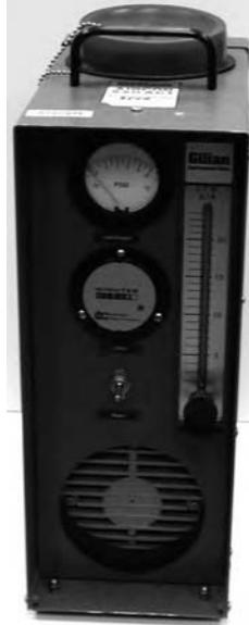
**FIGURE 64.8** High-volume sample pump.
