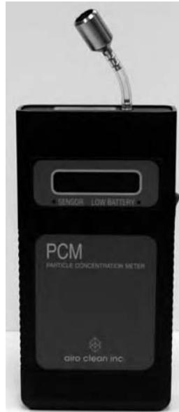
FIGURE 64.4 Direct-reading particle counter.
