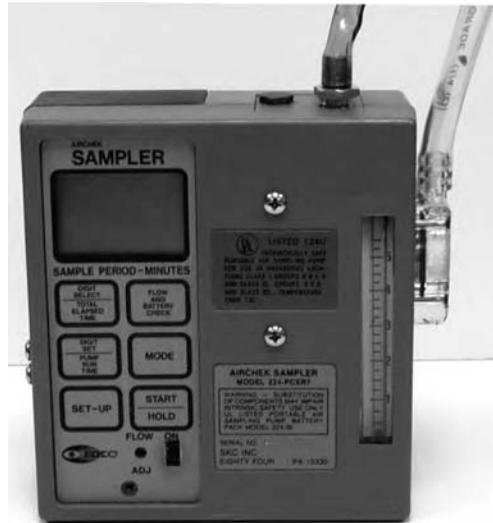
FIGURE 64.6 Low-volume programmable sample pump.
