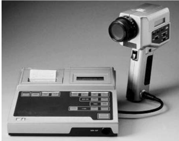
FIGURE 68.9 Luminance meter. (From Rea, M.S., Ed. [2000], IESNA Lighting Handbook: Reference and Application , 9th ed., Illuminating Engineering Society of North America, New York.)
