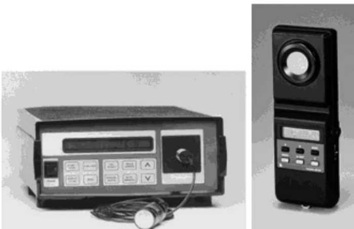
FIGURE 68.7 Illuminance meters. (From Rea, M.S., Ed. [2000], IESNA Lighting Handbook: Reference and Application , 9th ed., Illuminating Engineering Society of North America, New York.)
