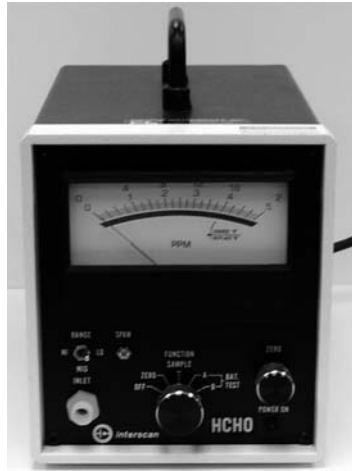
FIGURE 64.3 Direct-reading formaldehyde meter.
