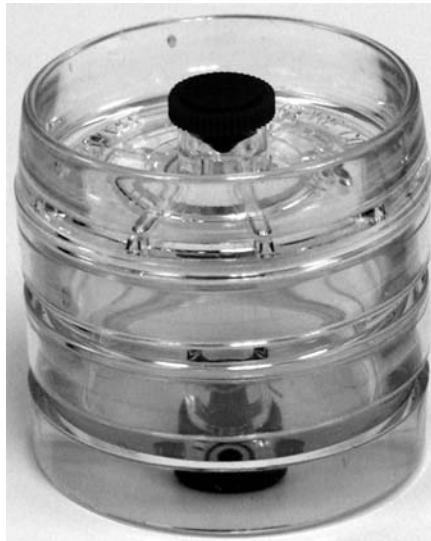
FIGURE 64.7 Filter cassette for collecting dust samples.
