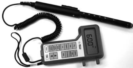
FIGURE 64.5 Multichannel IAQ monitor and data logger.
