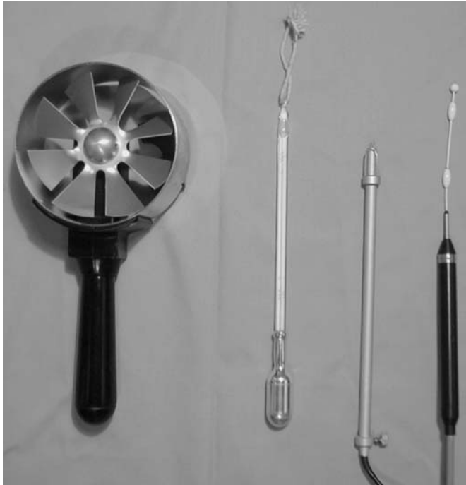
FIGURE 60.6 Sensors for air movement/wind: Vane anemometer (left), to be used in unidirectional air movement. Kata-thermometer (second from left), to be freely hanging in air after preheating. Cooling speed is related to air speed. Unidirectional hot wire anemometer (second from right): the actual wire protrudes at the top. It is extremely thin and is not really visible in this view. The shaft is used to protect the sensor when not in use. Spherical sensor (right), designed to be sensitive to multidirectional wind and with a fast response time.
