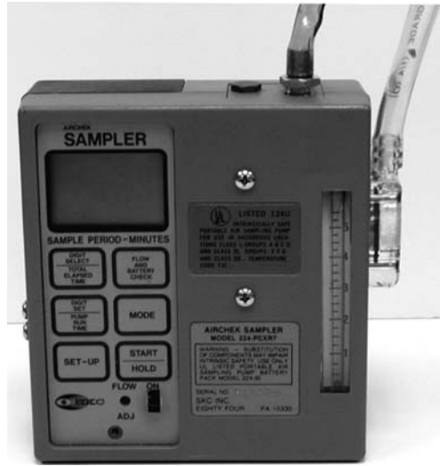
FIGURE 64.6 Low-volume programmable sample pump.
