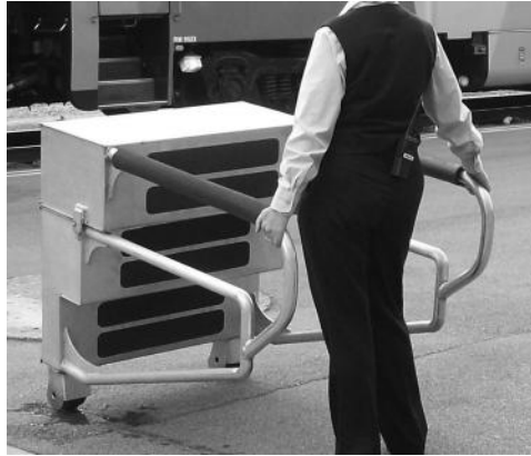
Figure 4.8 Portable stairs with handrails.
