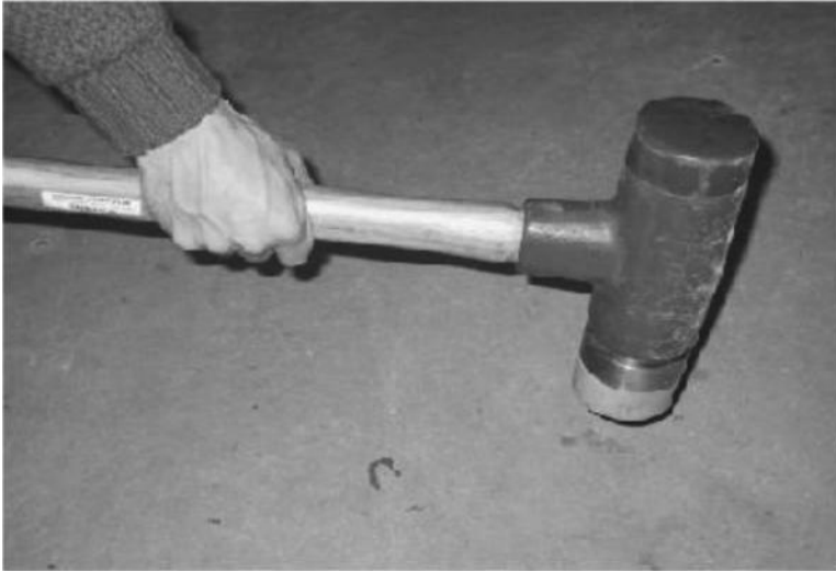
Figure 3.15 Power grip being used on a sledge hammer.
