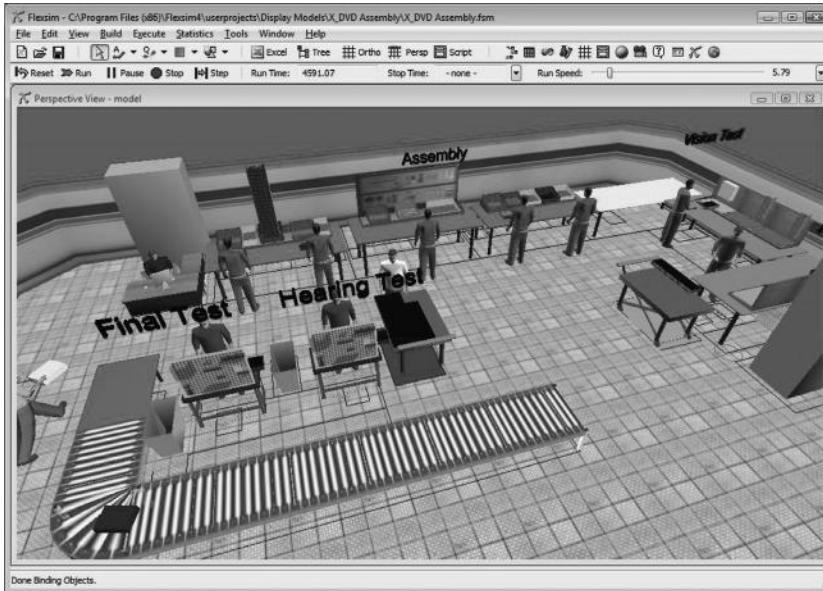
Figure 9.1 Example of work cell simulated using FlexSim. Simulated elements include the tasks performed by each operator at each station, movements of operators and product between stations, and work in progress (WIP).
