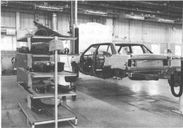
FIG. 6.12. Two-person work system at the Volvo Uddevalla plant.
