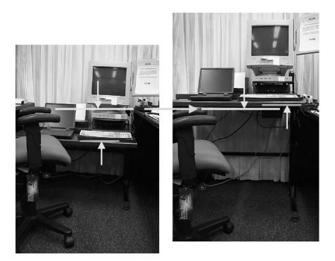
Figure 6-4 Office workstation showing range of adjustable heights.
