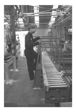
**Figure 6-9** Stair ladder installed on a conveyor line.
