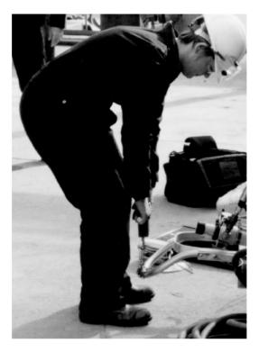
Figure 3-1 Using a force gauge to measure a pushing/pulling task.
