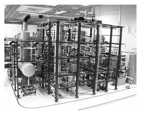
Figure 9-3 Plastic model used to illustrate the design of a chemical plant.
