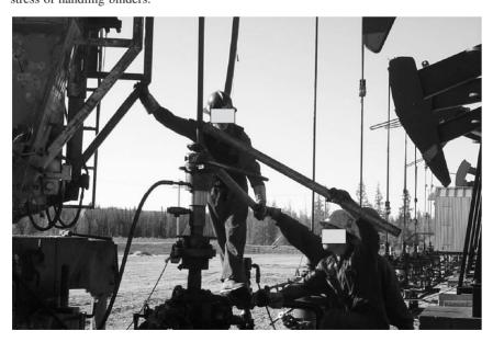
**Figure 6-19** Operator using an 8-ft extension to increase the force applied to a well-head block.
