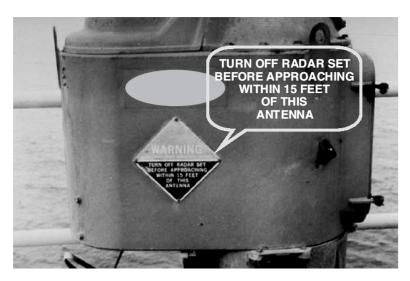
**Figure 2-2** Poor design of a warning sign; the text is too small to be read from 15 feet away.
