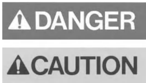
Figure 3 Examples of two signal word panels including alert symbol and color. Note that the DANGER panel is white print on red background and the CAUTION is black print on yellow background. Not shown is the WARNING panel, which is black print on orange background.
