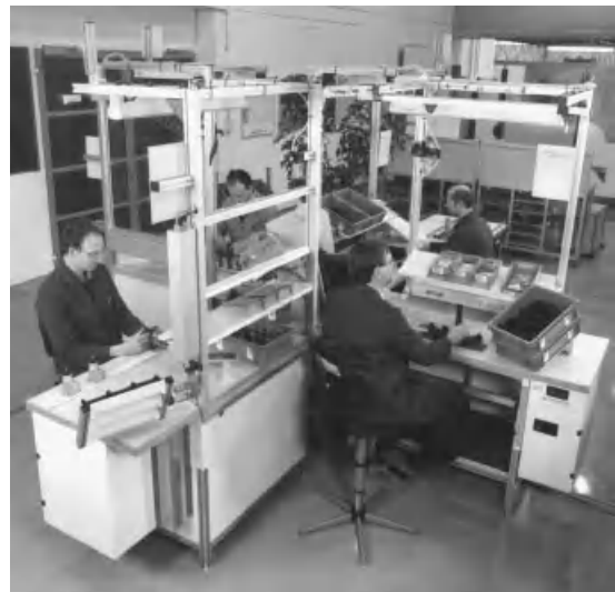
Figure 3 Group work assembly operation at an ergonomically optimized workstation. (Courtesy of Fraunhofer IAO.)
