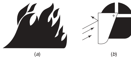
Figure 6 Examples of pictorials showing a direct representation: (a) raging fire and (b) wear eye shield.
