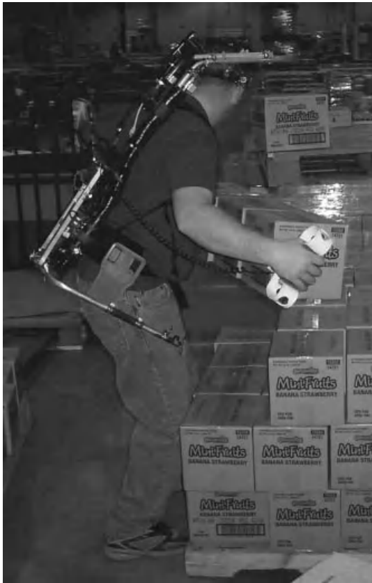
Figure 10 Moment monitor used to precisely measure exposure to dynamic load moments on the job.
