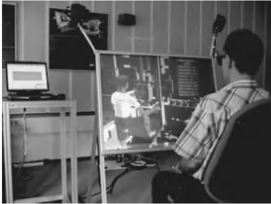
Figure 5 Anthropometric workplace design using the virtual human model ANTHROPOS on a Picasso-3D-Projection System. (Courtesy of Fraunhofer IAO.)
