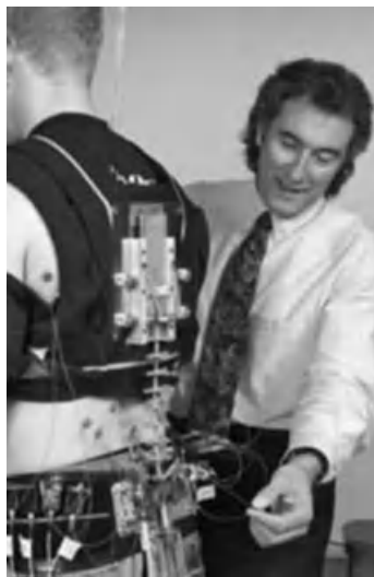
Figure 3 Marras’s lumbar motion monitor exoskeletal system enabling measures of the dynamic aspects of task. It captures information for calculation of the velocities and accelerations and angular velocities and angular accelerations that assist in predicting risk of lower back musculoskeletal injury (Marras, 2006).
