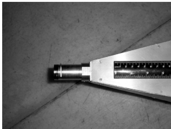
Figure 2. Ionization chamber with 2\text{ }\mu\text{g} ^{252}\text{Cf} source and preamplifier coupled to a pyramidal shielding, consisting from layers of iron, polythene and lead.
