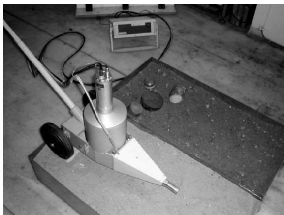
Figure 4. Geometry used in experiments with the prototype of mobile device for explosives detection with 2\ \mu\text{g}\ ^{252}\text{Cf} timed neutron source.
