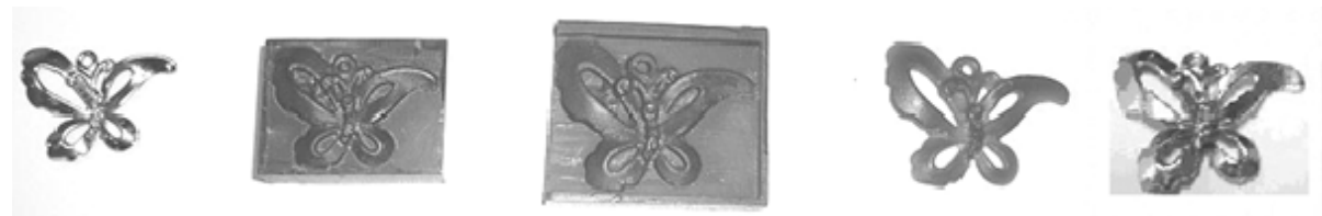
Figure 14. Wax jewel model manufactured through CNC micro-milling machine
