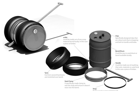
Figure 5. Open-ended problem solving exercise: water transportation for remote communities (Modular water transportation system for use in flooded landscapes (left); Water transportation system utilising readily available discarded materials (right))
