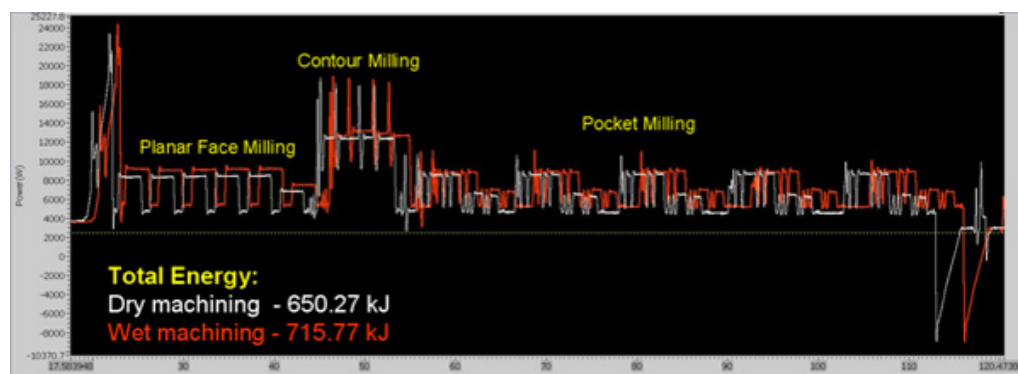
Figure 7. Machine tool system energy consumption (kJ) for part milling (wet vs. dry machining)
