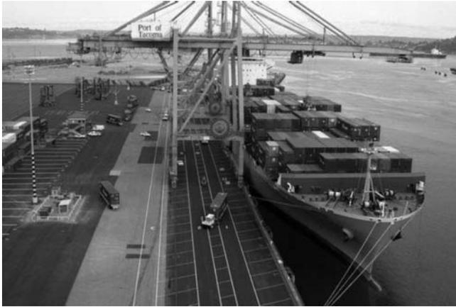
Figure 56.6 Ship to truck freight transfer.
