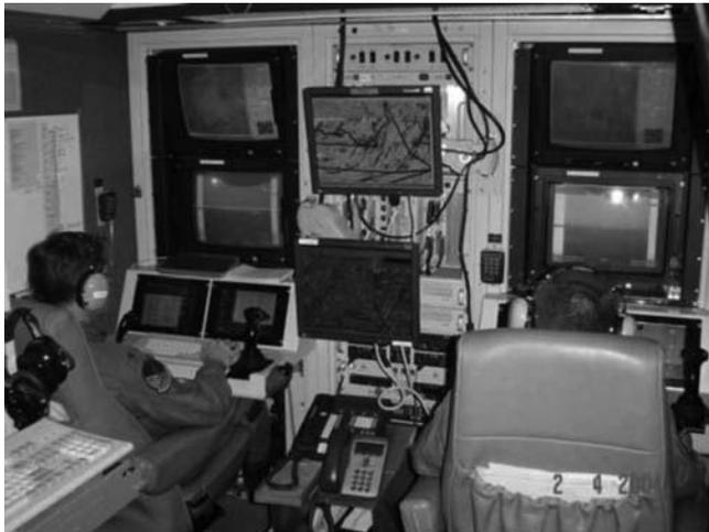
Figure 11.9 Current Predator UAS ground control station with pilot (left) and sensor operator (right).
