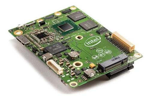
Figure 1-2. PCBA mounted with SOC and subsystems
