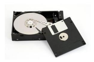
Figure 3-2. Magnetic storage devices
