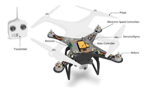
Figure 1-4. Parts of a drone
