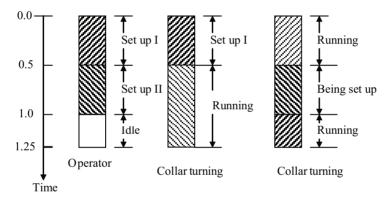
3.8 Man machine chart for one worker and two machines
