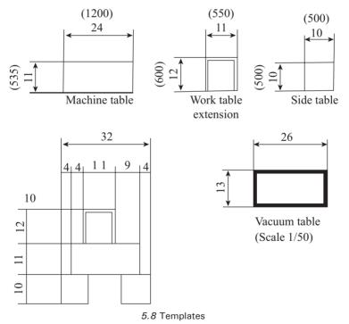
(5) Modify the layout according to the site limitations, including walls, pillars, and entry and exit locations for materials and finished goods.
