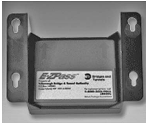
FIGURE 7.11 Mark IV roof mounted transponder.
