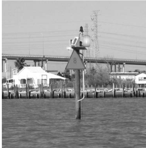
FIGURE 30.6 Modified navigational aid RFID marker portal.
