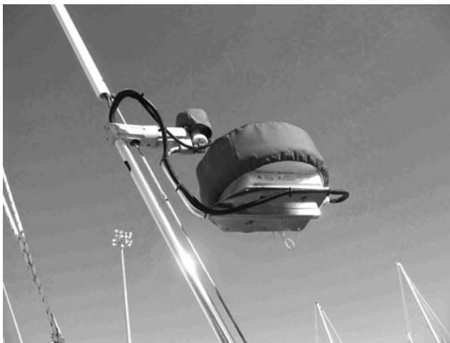
FIGURE 30.7 Questus hydraulically dampened antenna mount.
