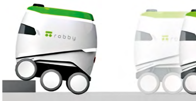
Figure 50: Robby Technologies Robby 2 can navigate autonomously with 6-wheel drive and advanced AI to handle obstacles and interaction with humans; Source: Robby.io
