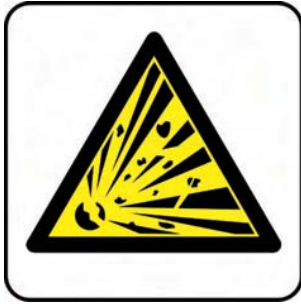
Figure 6.5 A typical explosive atmosphere warning sign
