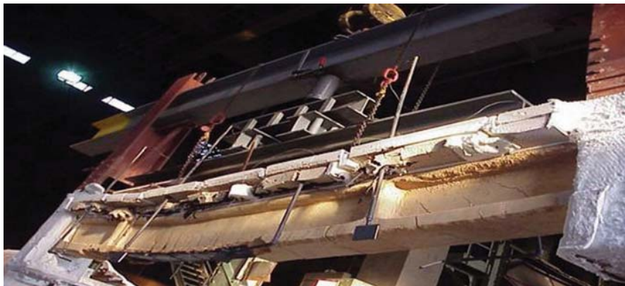
Figure 9.8 Structural beams having undergone fire tests
