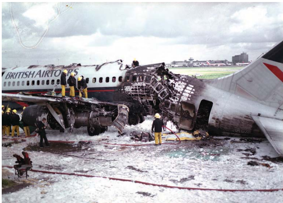
Figure 10.12 Manchester airport fire involving an aircraft on the runway – A quickly developing fire in an enclosed space which resulted in an urgent need to escape and reduced evacuation time
