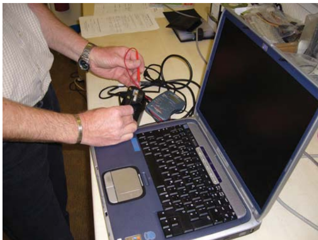
Figure 8.13 Portable appliance testing
