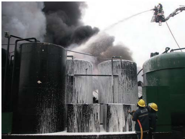
Figure 13.2 The use of fire fighting foam
