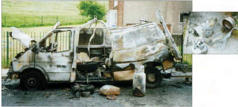
Figure 8.4 Van fire involving cylinders
