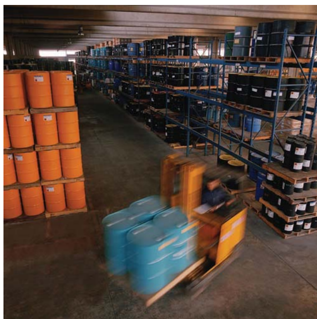
Figure 7.22 Example of fire load from storage containers in a warehouse
