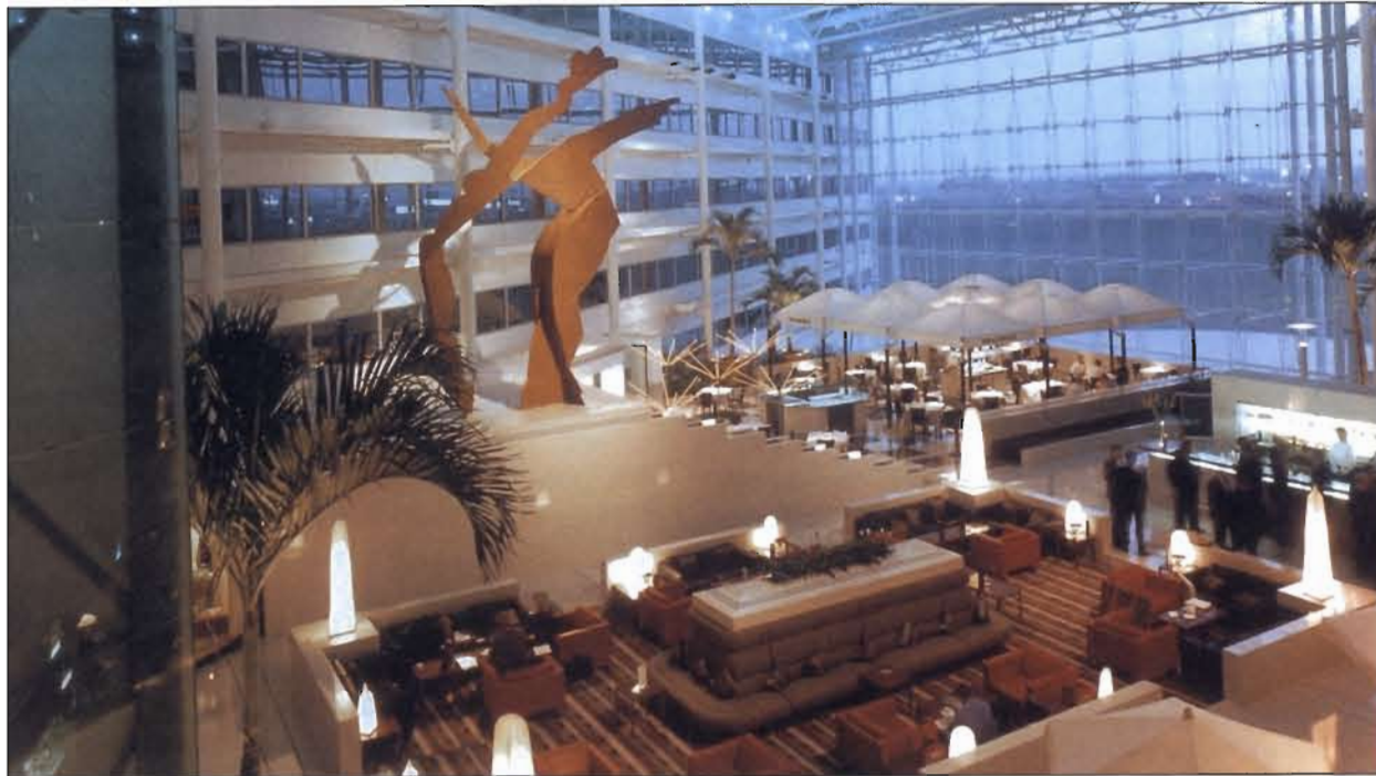
Figure 7.3 Interior of an ultra-modern hotel. The central lift shaft can be seen left. Note the fire detector left of the sculpture and unopenable windows to the atrium. Photo: Heathrow Sterling Hotel.
