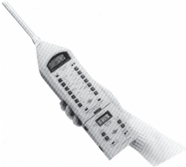
Figure 10b. A sound level meter and filter set for acoustic measurements
