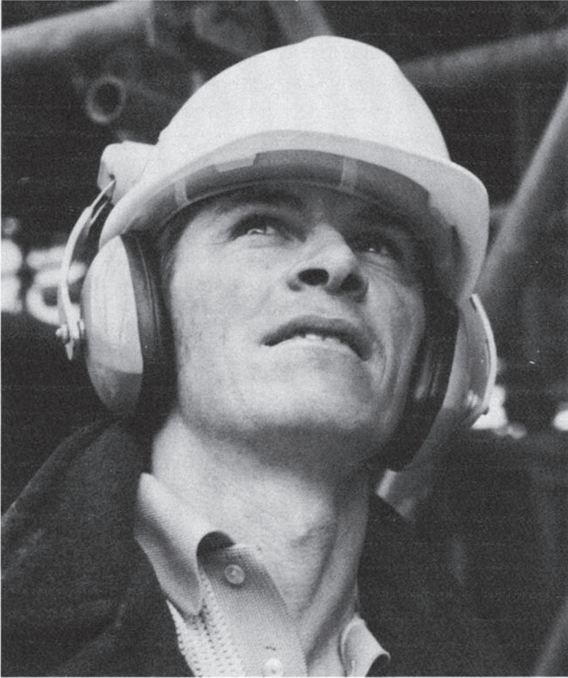
Plate 1. Muff type ear defenders. The version shown is fitted directly to the normal industrial safety helmet. Ear defenders should be used where noise levels exceed NR 85 or 90dBA
