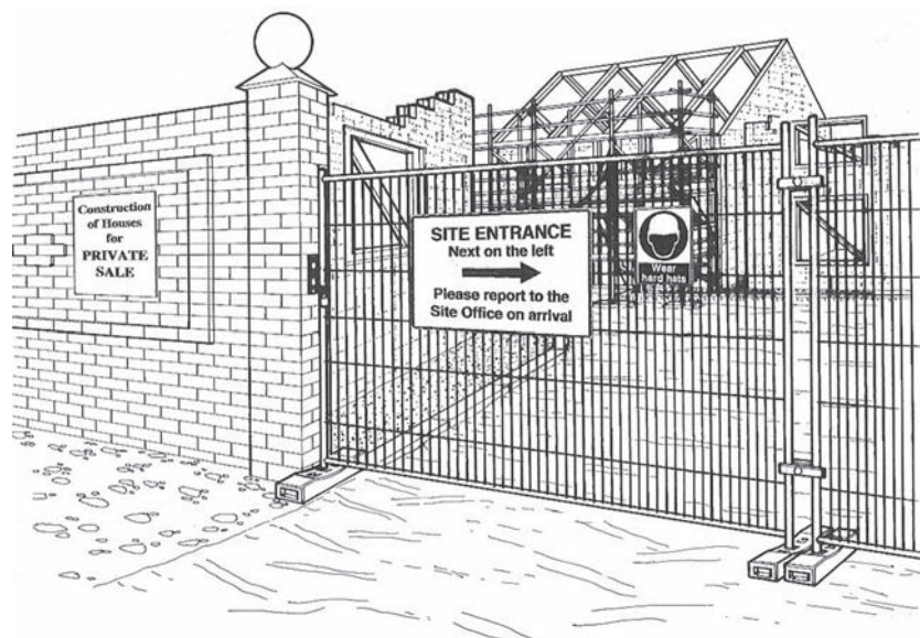
Figure 16.1 Secure site access gate.
