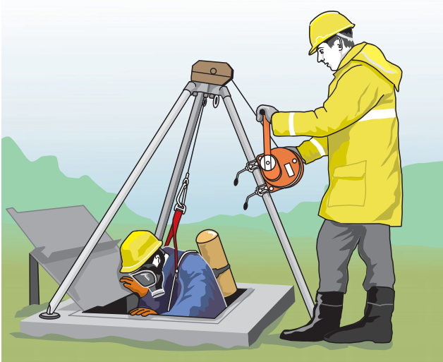
Figure 6.9 Entering a confined space.
