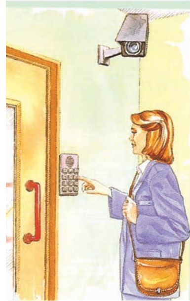
Figure 15.12 Security coded access and surveillance CCTV camera.
