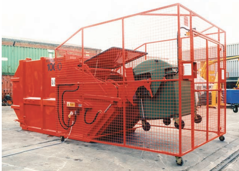
Figure 11.26 Typical retail compactor.
