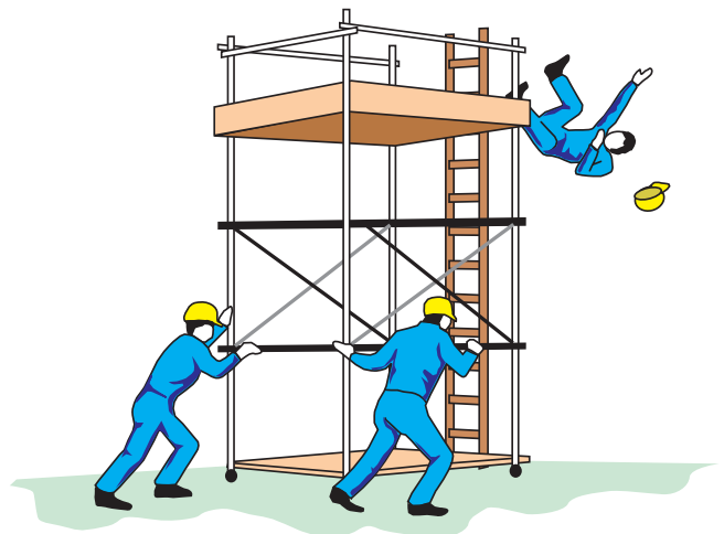
Figure 9.3 Falling from a height – tower scaffold.
