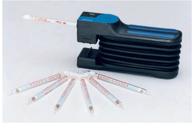
Figure 14.8 Hand pump and stain detector.
