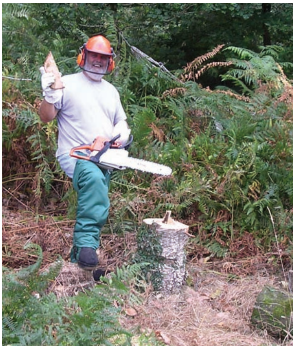
Figure 11.24 Kevlar gloves, over trousers and over shoes providing protection against chainsaw cuts. Helmet, ear and face shields protect the head. Apprentice under instruction – first felling.
