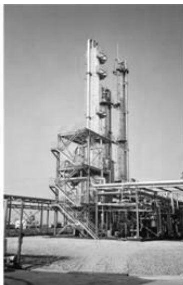
Figure 5.13. A. Example distillation column schematic Ref. 5.11, and B. typical industrial distillation column, ©Sulzer Chemtech Ltd.
