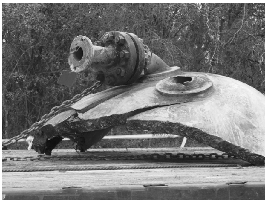
Figure 5.24. Portion of 3 inch thick reactor, Ref. 5.28.
