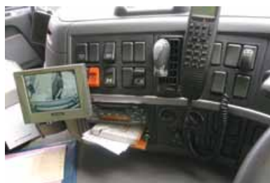
Figure 38 CCTV monitor in vehicle cab
