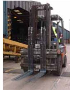
Figure 13 A lift truck passing through an interrupted road hump
