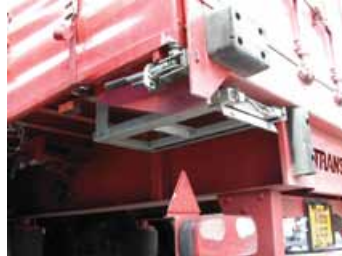
Figure 56 This LGV is fitted with a set of foldaway steps to make accessing the load easier
