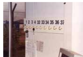
Figure 34 These hooks keep keys away from the vehicle until loading has been completed
