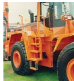
Figure 55 This piece of plant has a good access system, with steps and handholds. The first step is flexible to stop it being damaged in rough conditions
