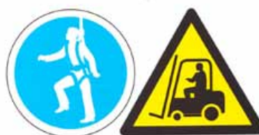
Figure 51 'Safety harnesses must be worn' and 'Industrial vehicles operating' signs
