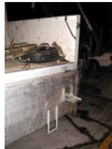
Figure 57 This dropside vehicle has been fitted with two footholds (one of which folds flat) and a handhold (not shown) to help workers access the load bed
