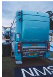
Figure 39 High centre-mounted CCTV camera
