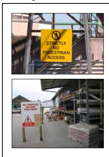
Figure 15 Examples of signs used to segregate pedestrians and vehicles
