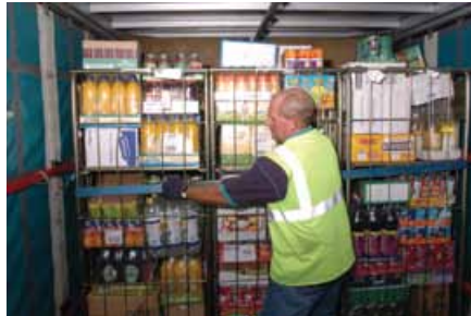
Figure 47 Securing rollcages in a curtainslider
