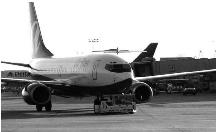
**Figure 16.8** A tow tug towing AirTran's 737-700 aircraft
