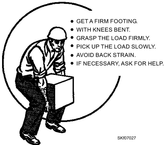
Figure 7-27. —An example of manual lifting.
