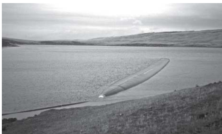
The dracone was invaluable for keeping a supply of fuel near shore. All but this one were lost on the Atlantic Conveyor . (Courtesy Robin Smith)
