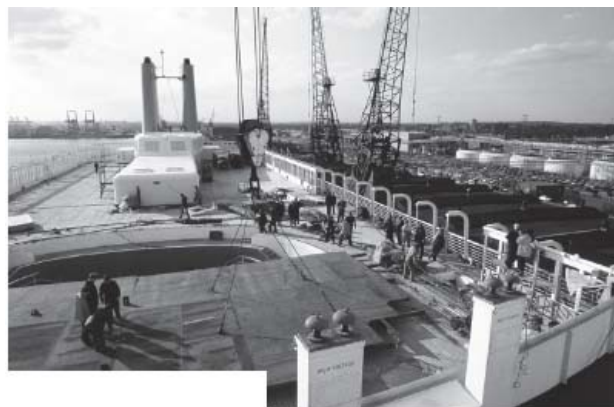
Workers install a flight deck atop the swimming pool of Canberra . The ship with many modifications sailed loaded with troops three days after arriving in Southampton. (Courtesy P&O Heritage Collection)
