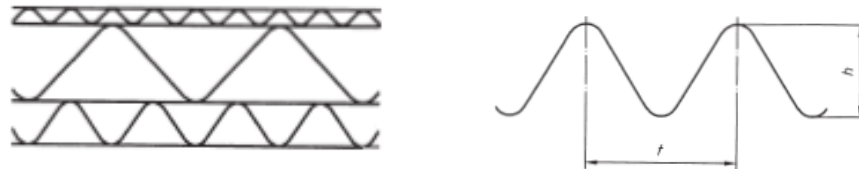
Figure 7.2-1: Triple-wall corrugated fiberboard (left) and Flute dimension (right)
