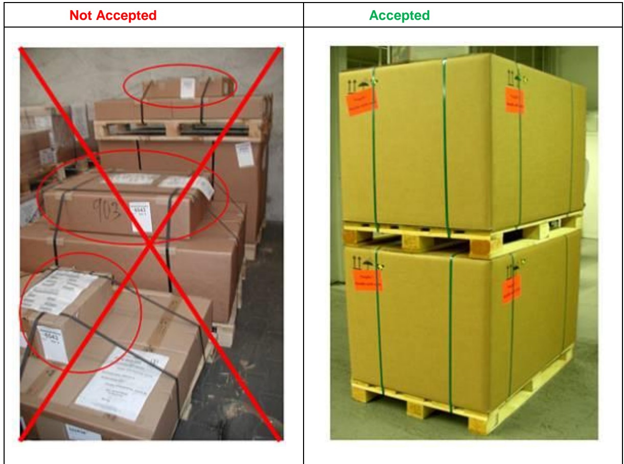
Figure 7.2-2: Not accepted and accepted loading units (LU)
