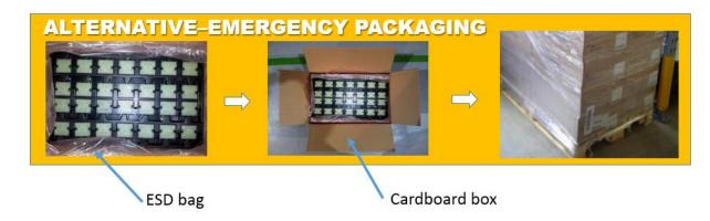
Figure 5.4-2: Example of alternative non ESD cardboard box (with ESD plastic tray and ESD bag)
