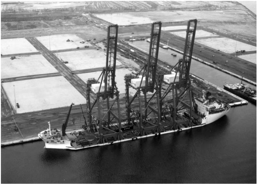
Figure 4-4 A heavy-lift ship carrying three container cranes, each 112 meters high and with sufficient reach to handle container ships 22 containers across. (Courtesy Amsterdam Port Authority.)
