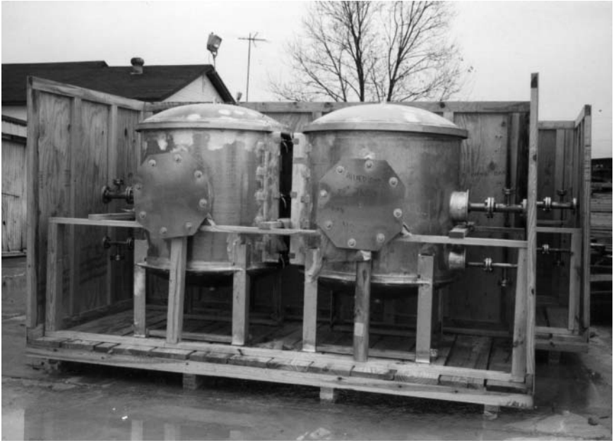
Figure 13-3 Export packer's protective crating for plastics refinery equipment. Courtesy of Superior Packing Inc./HAL, Inc.
