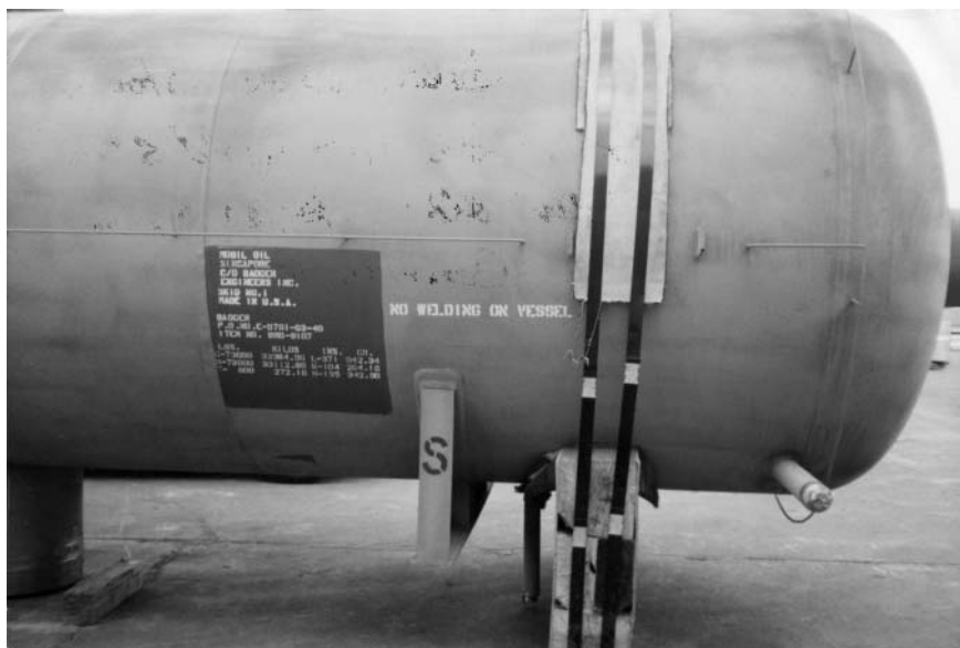
Figure 6-4 Tank destined for export, showing weight in pounds and kilos and dimensions in inches and centimeters. Courtesy of Superior Packing, Inc. HAL, Inc.
