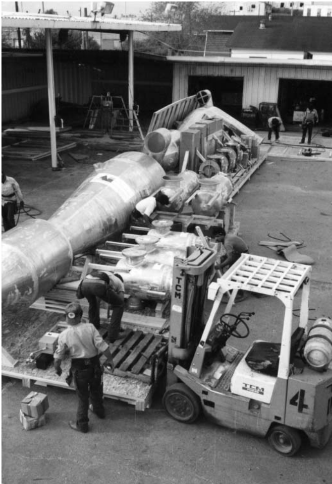
Figure 13–2 Export packer building protective crating around plastics refinery equipment. Courtesy of Superior Packing Inc./HAL, Inc.
