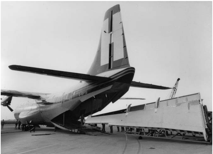
Figure 14–2 Airplane wing being loaded for delivery. (Photo courtesy of Heavylift Cargo Airlines.)
