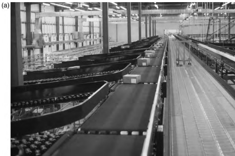
FIGURE 11.8 Various conveyors types and their applications in material movement and sortation (a–d). (Courtesy of FKI Logistex, Dematic Corporation. With permission.)
