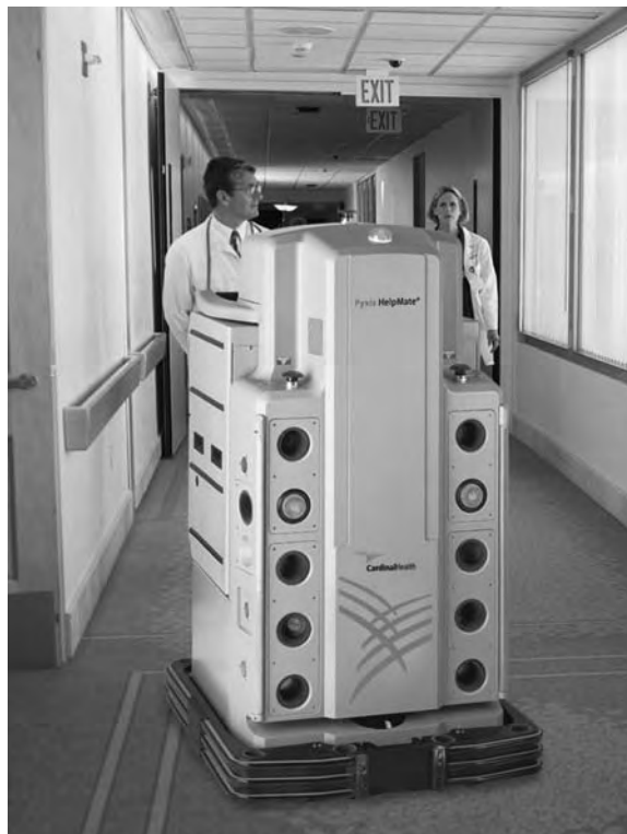
FIGURE 29.3 The Pyxis HelpMate® robotic courier.
