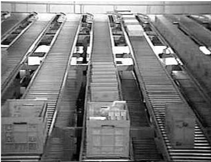
FIGURE 11.2 Gravity roller conveyor. (Courtesy of Sunderesh S. Heragu, 10 Principles of Materials Handling, CD. With permission.)
