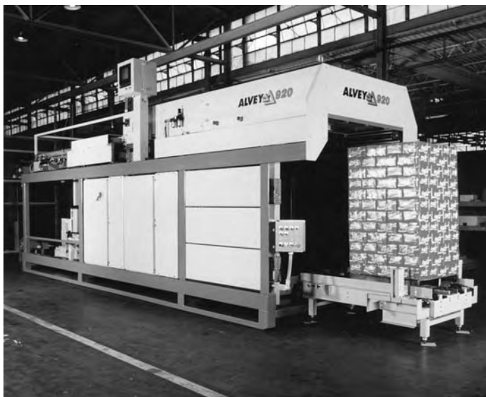
FIGURE 11.9 Palletizer. (Courtesy of FKI Logistex, Dematic Corporation. With permission.)
