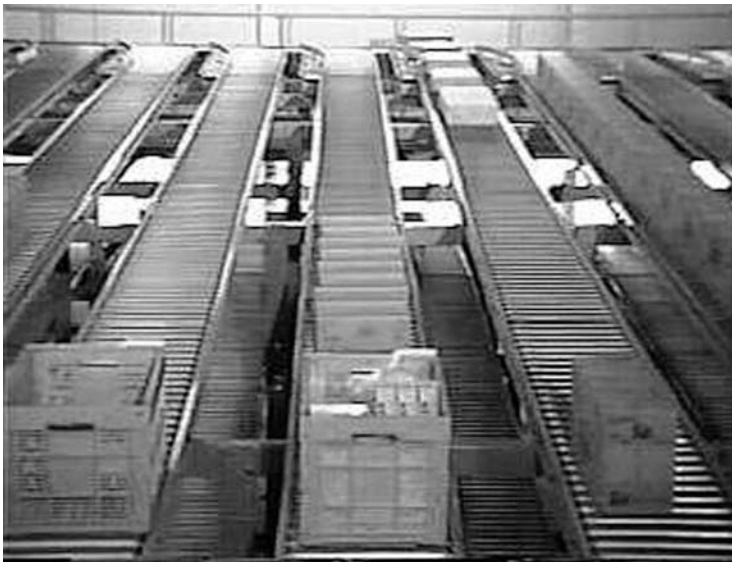
FIGURE 7.2 Gravity roller conveyor. (Courtesy of Sunderesh S. Heragu, 10 Principles of Materials Handling, CD. With permission.)
