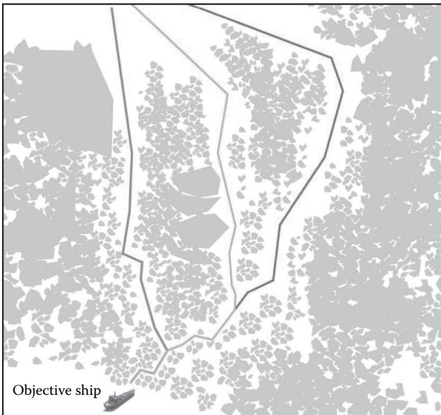
**Figure 5.3** Routes for the ship navigation in ice-covered sea regions (tracks 1, 2, and 3 from left to right).
