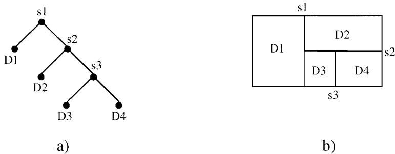
Figure 5.5. Example of a slicing tree and the corresponding block layout
