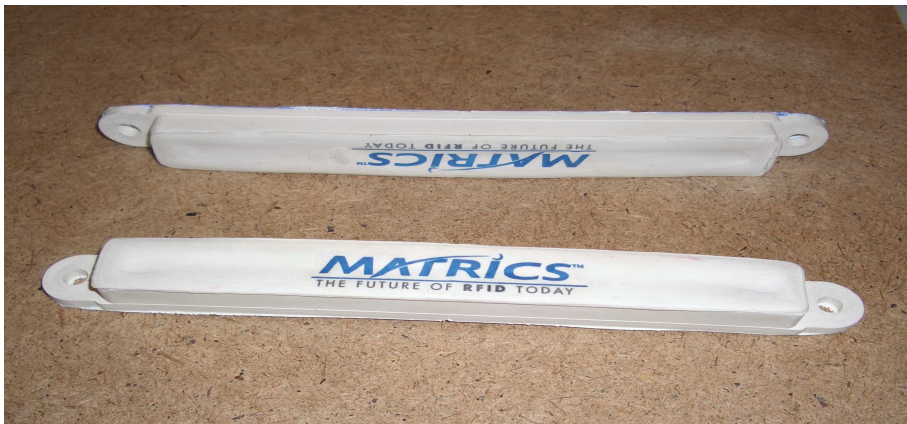
Figure 3. The EPC class 0 tag of model; Matrics i1010.
