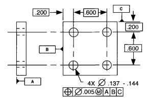
The  $\mathbb{W}$  in the feature control frame invokes the MMC concept and allows an increase in the amount of positional tolerance as the features depart from the maximum material condition.
