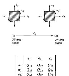
The transformation of on-axis unidirectional properties to off-axis is given by
