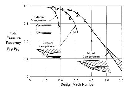
The figure illustrates the achievable pressure recovery trends with design flight Mach number for each of the inlet types. Although the mixed compression inlet provides higher recovery at supersonic conditions, its increased weight, increased control complexity, and increased bleed requirements must be balanced against the improved supersonic recovery. For a multi-mission aircraft, this is seldom a favorable trade.
