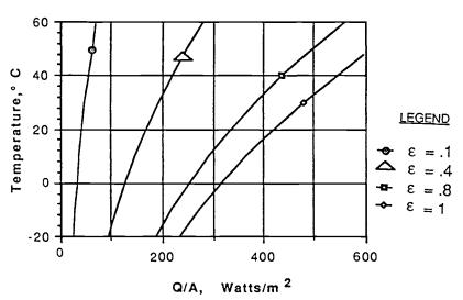
$$\sigma \epsilon_S A_S T_S^4 = \sigma \epsilon_S F_{S,E} A_S T_E^4 + \dot{Q}_S + \dot{Q}_{ER^*} + \dot{Q}_1$$
