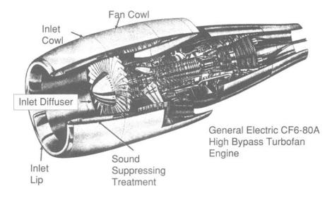
A nacelle and engine cross section is shown to delineate the nacelle component nomenclature. The major components of the nacelle and their functions are as follows: 1) inlet, to provide air to fan with acceptable flow qualities; 2) fan exhaust nozzle, to accelerate flow to produce thrust; 3) core exhaust nozzle, to accelerate flow to produce thrust; reverser, to decelerate aircraft during landing and rejected takeoff.
