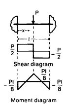
$V_x = V = \pm \frac{P}{2}$   $M_x = P\left(\frac{x}{2} - \frac{l}{8}\right) \quad \left(\text{when } x < \frac{l}{2}\right)$   $M_x = -\frac{Pl}{8} \quad \left(\text{when } \frac{x = 0}{x = l}\right)$   $M = +\frac{Pl}{8} \quad (\text{at center of span})$   $y = \frac{Pl^3}{192EI}$
