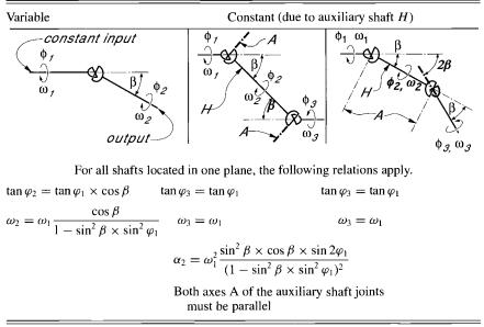
Note: The more the angle of inclination  $\beta$  increases, the more the maximum acceleration  $\alpha$  and the accelerating moment  $M_{\alpha}$  become; therefore, in practice,  $\beta \leq 45$  deg.
