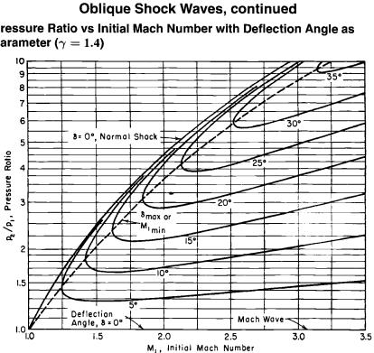
Pressure Ratio vs Initial Mach Number with Deflection Angle as Parameter ( $\gamma = 1.4$ )
