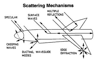
Most scattering levels relative to the peak RCS may be quite small but, away from the peaks, scattering due to these mechanisms can dominate. The scattering mechanisms are described in the following sections.
