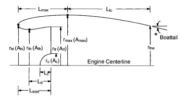
The following are the most significant geometric parameters and their major influence factors used in describing a particular inlet design. These parameters have been determined from the results of an experimental database, flowfield analysis, and wind tunnel testing.
