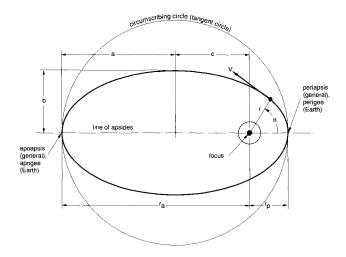
e = eccentricity =  $c/a = (r_a - r_p)/(r_a + r_p)$   $V = \sqrt{(2\mu/r) - (\mu/a)}$  *n* = mean motion =  $\sqrt{\mu/a^3}$  (angular velocity the spacecraft would have if traveling on a tangent circle instead of the ellipse)
