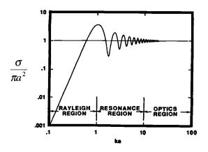
RCS of a metallic sphere with radius of *a*. (Source: *Radar Cross Section*, page 53, figure 3-5, by Knott, Schaeffer, and Tuley. Copyright ©1985, Artech House Publishers, Norwood, MA. Reproduced with permission of Artech House, www.artechhouse.com.)
