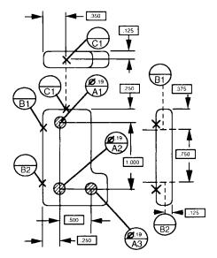
Typical drawing callout using datum targets to establish a datum reference frame for all three axes.
