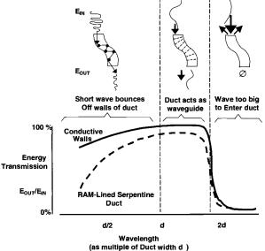
Duct scattering mechanism as a function of wavelength. (Source: Aviation Week and Space Technology, March 19, 2001. Reproduced with permission.)
