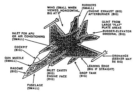
Standard jet fighter aircraft design with scattering sources indicated. (Source: *Radar Cross Section Lectures*, by A. E. Fuhs. Copyright ©1984, AIAA, New York. All rights reserved. Reprinted with permission of AIAA.
