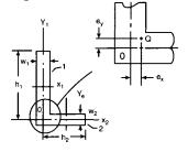
Leg 1 = rectangle  $w_1h_1$ ; leg 2 = rectangle  $w_2h_2$  $I_1$  = moment of inertia of leg 1 about  $Y_1$  (central axis)  $I_2$  = moment of inertia of leg 2 about  $Y_2$  (central axis)
