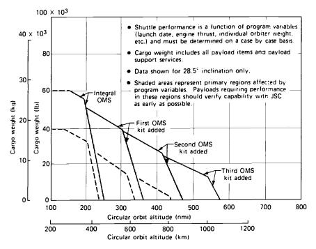
Near-term Space Shuttle cargo weight vs circular orbital altitude-KSC launch
