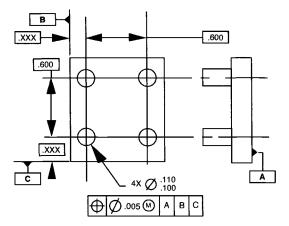
Part 2-Fixed studs. (Inserts, pins, fixed nut plates, countersunk holes.)
