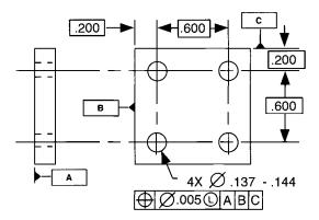
The ① in the feature control frame invokes the LMC concept and allows an increase in the amount of positional tolerance as the features depart from the least material condition. Note: This example, which is used to demonstrate the least material condition would hardly ever be seen in real practice. Replacement of the four holes with a shaft of the same diameter would be more typical.
