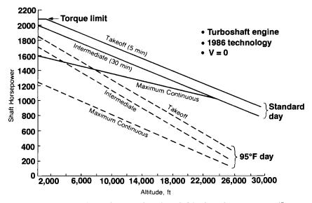
Typical uninstalled engine ratings as a function of altitude and temperature. (Source: *Helicopter Performance, Stability, and Control*, page 274, figure 4.1, by R. W. Prouty. Copyright © 1995, Krieger Publishing Company, Malabar, FL. Reproduced with permission of Krieger.)
