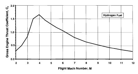
Ramjet Gross Thrust Coefficient vs Mach number
