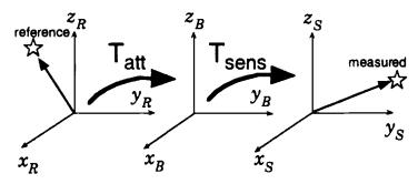
Measurements of reference vectors (e.g., sun, stars, local vertical) made in the sensor frame are used to compute the attitude matrix  $T_{\text{att}}$ .  $T_{\text{att}}$  is usually parameterized in Euler angles for analysis or Euler symmetric parameters (quaternions) for numerical computations.
