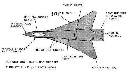
Stealthy jet fighter aircraft design with RCS reduction guidelines incorporated. (Source: *Radar Cross Section Lectures*, by A. E. Fuhs. Copyright ©1984, AIAA, New York. All rights reserved. Reprinted with permission of AIAA.
