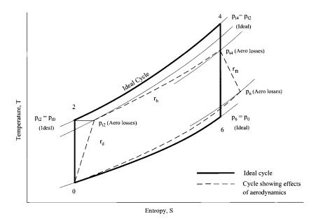
The figure shows the effects of aerodynamic losses on a temperature–entropy (T–S) diagram where the processes are no longer isentropic, thereby resulting in entropy changes.
