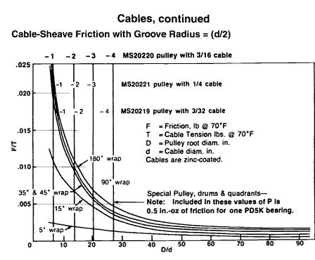
Cable-Sheave Friction with Groove Radius = (d/2) + 0.02
