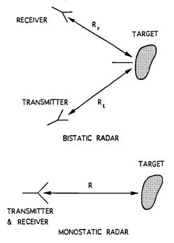
Bistatic cross section is defined as the scattering cross section in any specified direction other than back toward the source. In most applications, the transmitter and receiver are located on the same platform and frequently share the same antenna. In this case the radar is monostatic. Monostatic cross section or back scattering cross section is defined as the scattering cross section in the direction toward the source.
