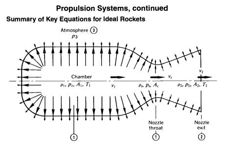
Note: Four subscripts are used above (1, 2, 3, t). They are shown in circles and refer to the specific locations. Thus,  $p_1$  is the chamber pressure,  $p_2$  is the nozzle exit pressure,  $p_3$  is the external fluid of atmospheric pressure, and  $p_t$  is the nozzle throat pressure.  $T_1$  is the combustion chamber absolute temperature.
