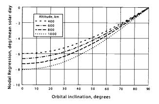
Nodes move westward for direct orbits (0 deg  $\leq i \leq 90$  deg) and eastward for retrograde orbits (90 deg  $\leq i \leq 180$  deg).
