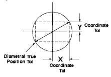
This conversion may only be used if the designer takes into account the tolerance across corners of a square zone. If not, a conversion of this type could result in a round tolerance zone much larger than is really allowed.
