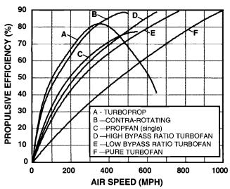
**Propulsive Efficiency vs Airspeed**
