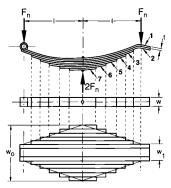
The calculation does not consider friction. In practice, friction increases the carrying capacity by between 2 and 12%.
