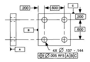
The absence of a feature control symbol in the feature control frame invokes the RFS concept and allows no increase in the amount of positional tolerance as the features depart from the maximum material condition. Note: If nothing appears in the feature control frame following the tolerance, then the RFS condition is assumed.
