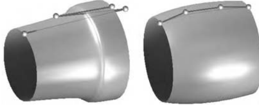
FIGURE 4.4 Hub and shroud geometry for axial compressor example.
