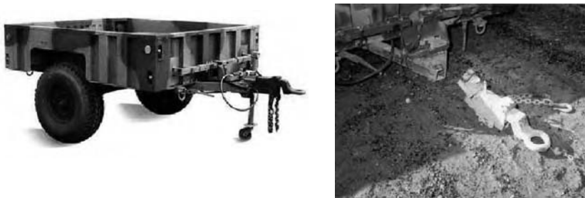
FIGURE 8.3 Army trailer and its structural failure.
