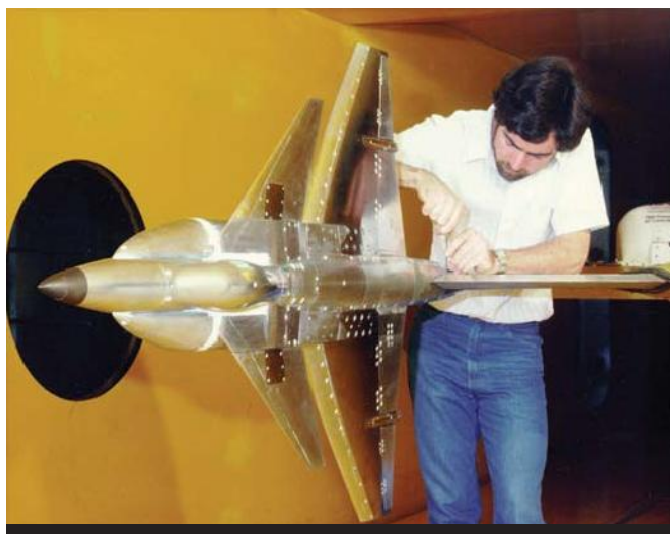
A NASA engineer mounts a model of one of the iterations of the McDonnell Douglas Model 279, a supersonic lift-cruise vectored thrust aircraft with a close-coupled canard/tailess delta layout, in a wind tunnel at NASA's Ames Research Center. The Model 279 was one of many STOVL designs analyzed over the years for programs that eventually died out or merged into the JSF program.
