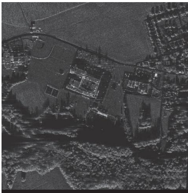
A synthetic aperture radar (SAR) image from the F-35’s AN/APG-81 Active Electronically Scanned Array (AESA) radar. Because an AESA radar uses many small radiating and receiving elements rather than a single dish, sections of the radar can be devoted to different tasks. While the radar can produce high-fidelity SAR images of a target area, for example, it can also be working in an air-to-air mode.
