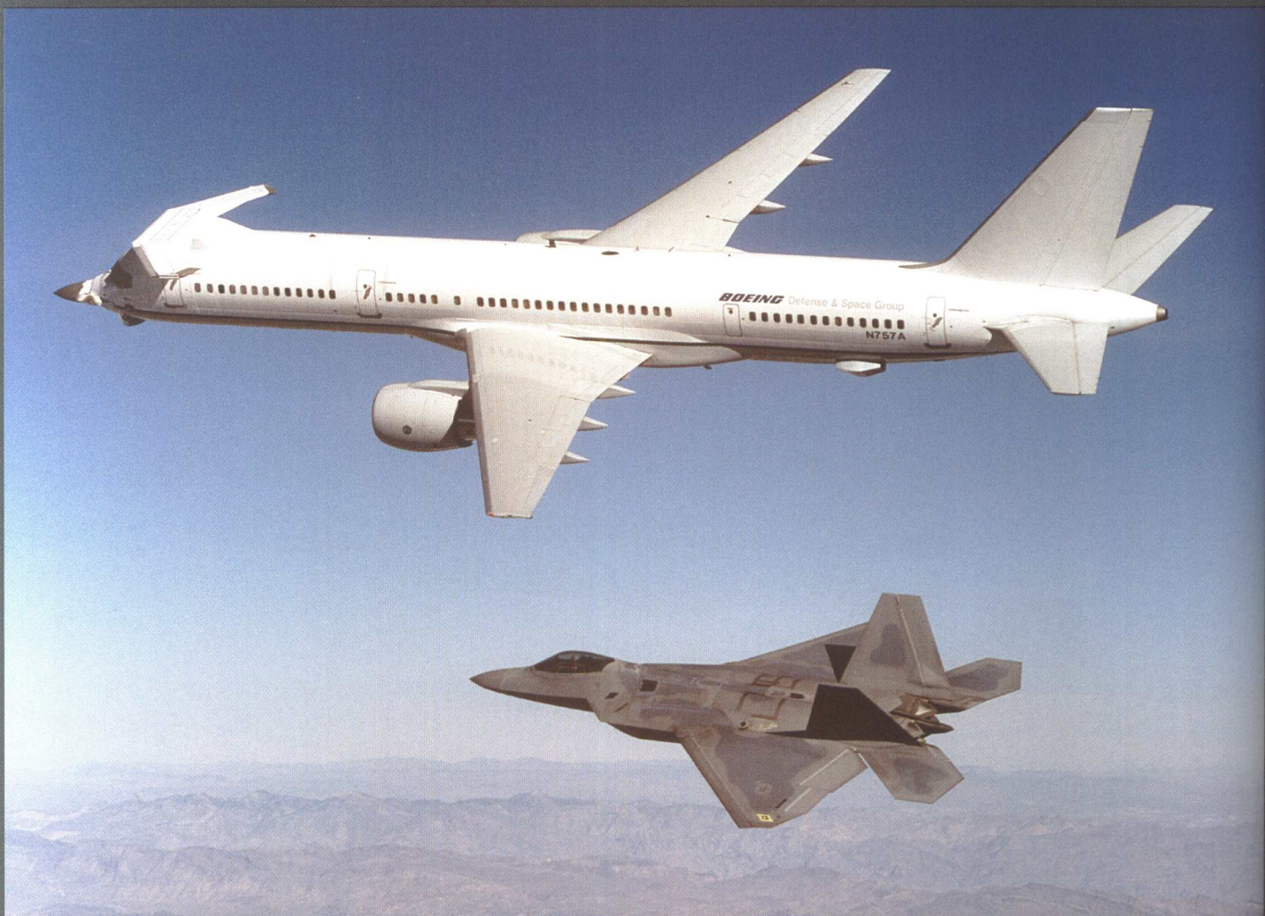
Boeing's prototype 757, N757A, served as a flying laboratory for the YF-22A and F/A-22A avionics and weapon systems.
