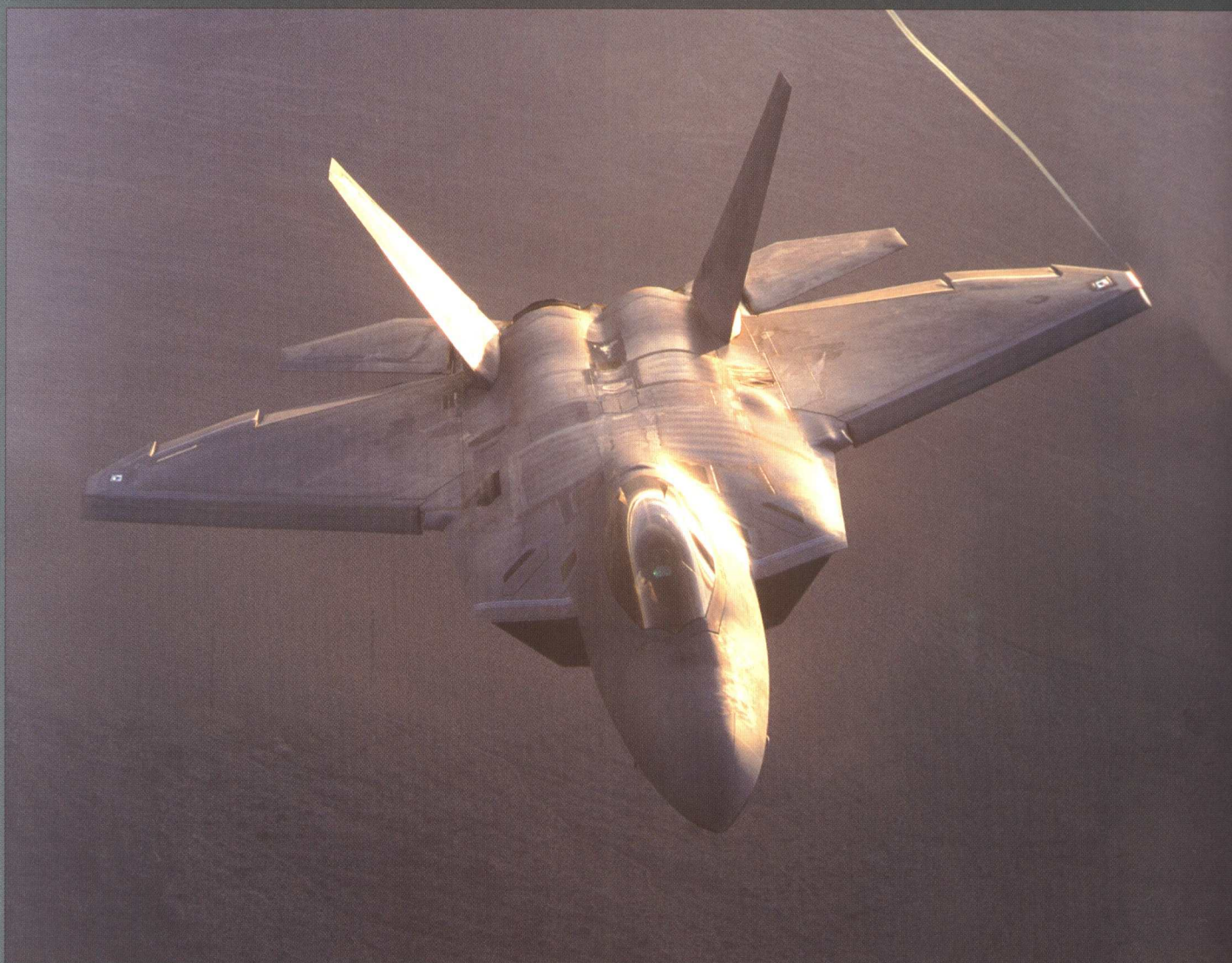
An unidentified EMD F/A-22A over the Edwards test range. Deflected full-span leading edge flaps are noteworthy.
