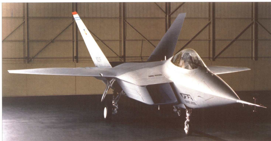
Above: YF-22A full-scale pole model at Lockheed Martin's Helendale, California radar cross section test facility. Lockheed Martin
