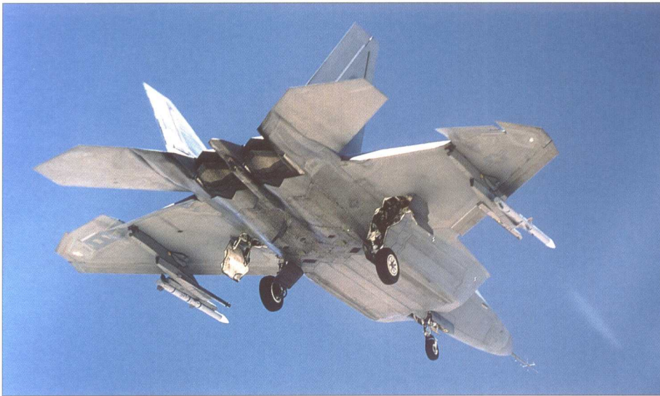
Top: F/A-22A has been cleared for external carriage of AIM-9 and AIM-120. Lockheed Martin
