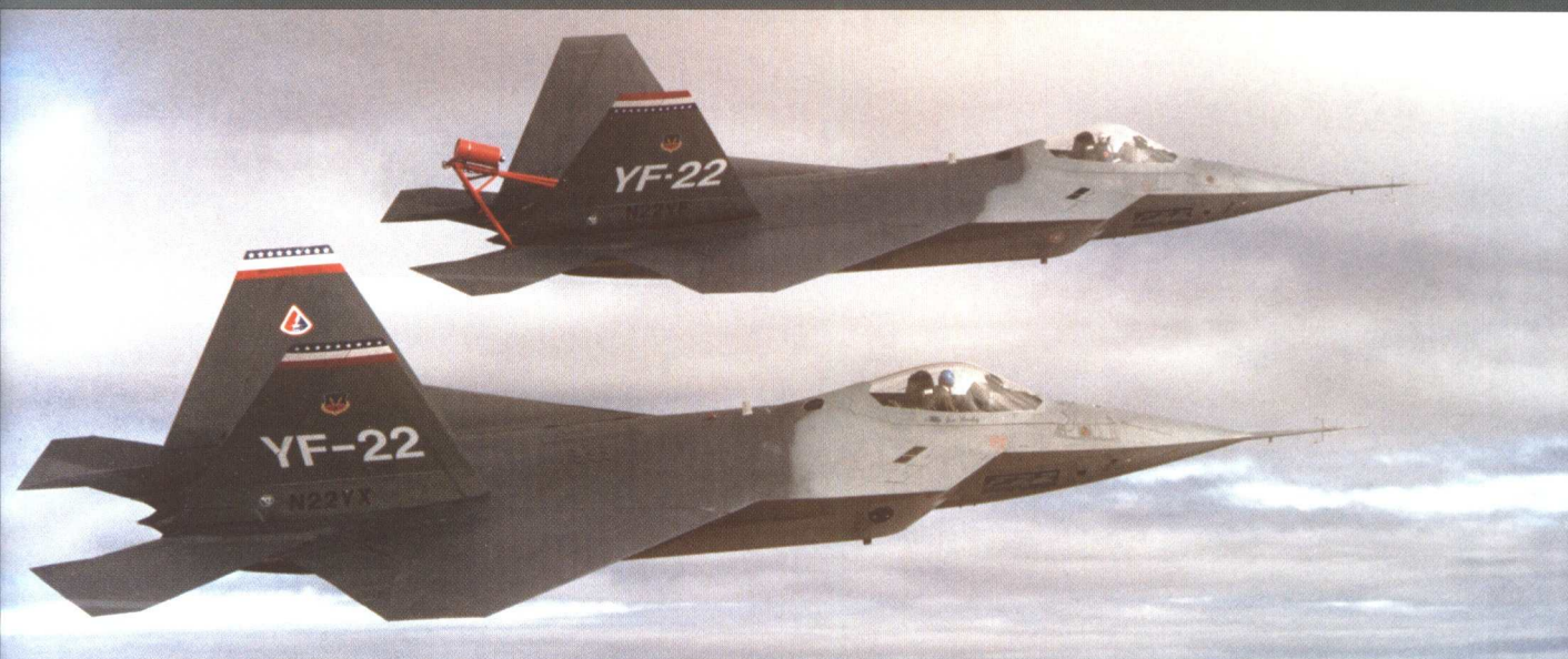
Pratt & Whitney YF119 -PW-100-powered YF-22A, N22YX (foreground) and General Electric YF120-GE-100 -powered YF-22A, N22YF.
