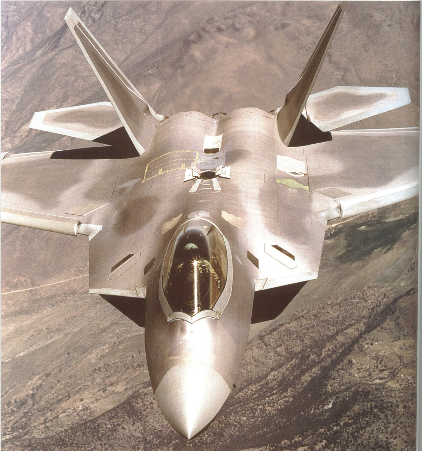
Below: Unidentified F/A-22A moves in for inflight refueling session behind a Boeing KC-135R. Noteworthy is open refueling receptacle which is normally covered by two mechanically actuated and low-observables optimized doors. Lockheed Martin
