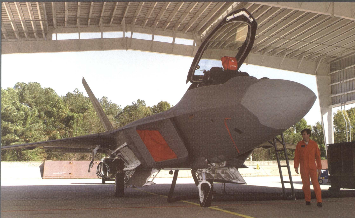
F/A-22A, 02-4032, during ground inspection and prior to static engine run in bay at Lockheed Martin's Marietta, Georgia facility.
