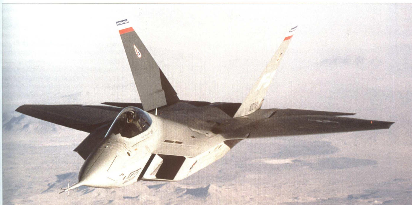
Below: YF-22A, N22YX, over Edwards during Dem/Val tests. Full-span leading edge flaps are readily discernible. Lockheed Martin
