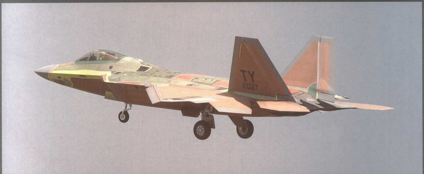
F/A-22A, 01-4027, sans paint. It has since been delivered to Tyndall AFB, Florida. Various radar absorbent panels are readily discernible.
