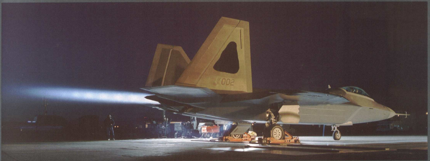
Second EMD F/A-22A, 91-4002, undergoing static engine run at night.
