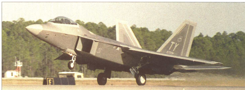
Right: F/A-22A, 02-4031, immediately following touchdown at Tyndall AFB. The F/A-22A uses its toed-in rudders as airbrakes. The aircraft is not equipped with a drag chute. Norm Taylor
