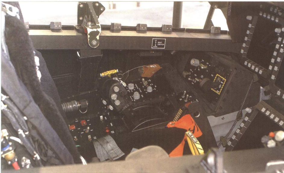
Top: F/A-22A left console includes throttles and landing gear extension/retraction handle.
