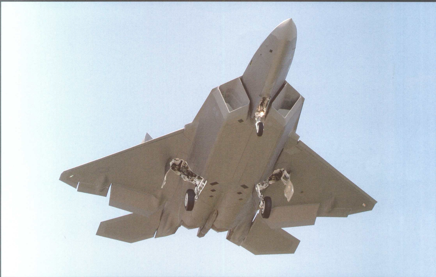
F/A-22A, 01-4025, on final to Marietta, Georgia and prior to delivery to Nellis AFB. Tailhook fairing is readily visible between engine nacelles.
