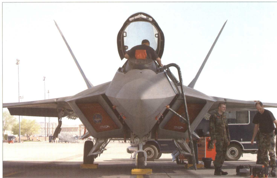
Right: Angular nose radome cross-section is the end product of low-observables requirements. Jay Miller
