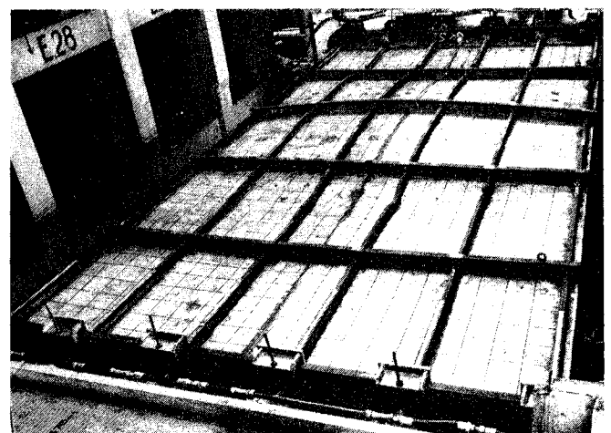
(c) OVERALL GRILLAGE BUCKLING (MODE 4)
