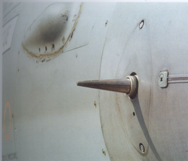
Top: Left and right view on the Angle Of Attack (AOA) probes on the Viper's nose.
