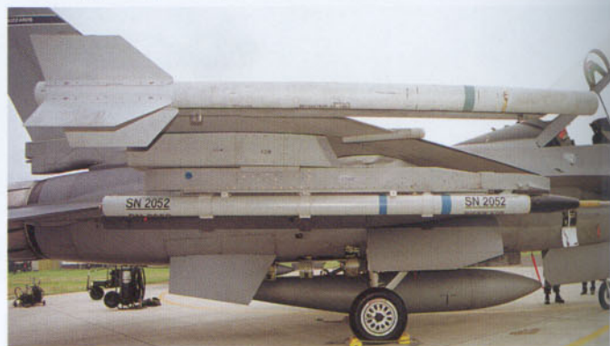
Below: The F-16 is stealthier than you might think, due to the Radar-reflecting paint applied. Ground radars have difficulties to interpret the right location of an F-16 on their screens, which can be dangerous for civilian aircraft. The AMA has a Radar Reflecting metal head mounted on the tube of the Sidewinder, and gives the right location of the F-16 during peace time. Normally it is always placed on Station 9, the right hand side wing tip station.
