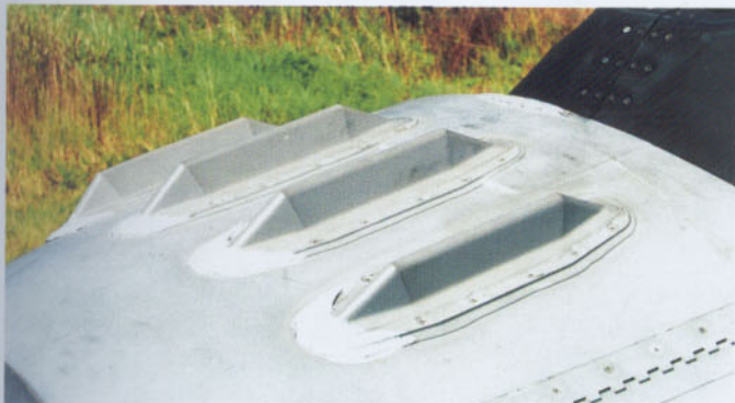
Below and right: Belgium, the Netherlands, Denmark, Norway and Portugal have updated most of their F-16s to MLU standards, and one of the new features are the Advanced IFF antennas just in front of the canopy.
