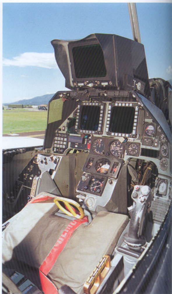
One difference between the single and the two seat F-16s, is the air conditioning grid. In the latter, do not have the box-shaped grids. Note the detail of the canopy framing in this photo.
