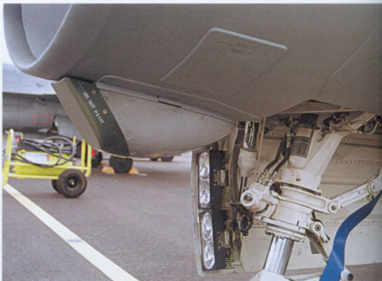
Below & left: Details of the CARAPACE - ECM pod, only to be found on Belgian F-16s.
