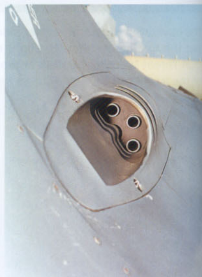
Below & left: Details of the CARAPACE - ECM pod, only to be found on Belgian F-16s.
