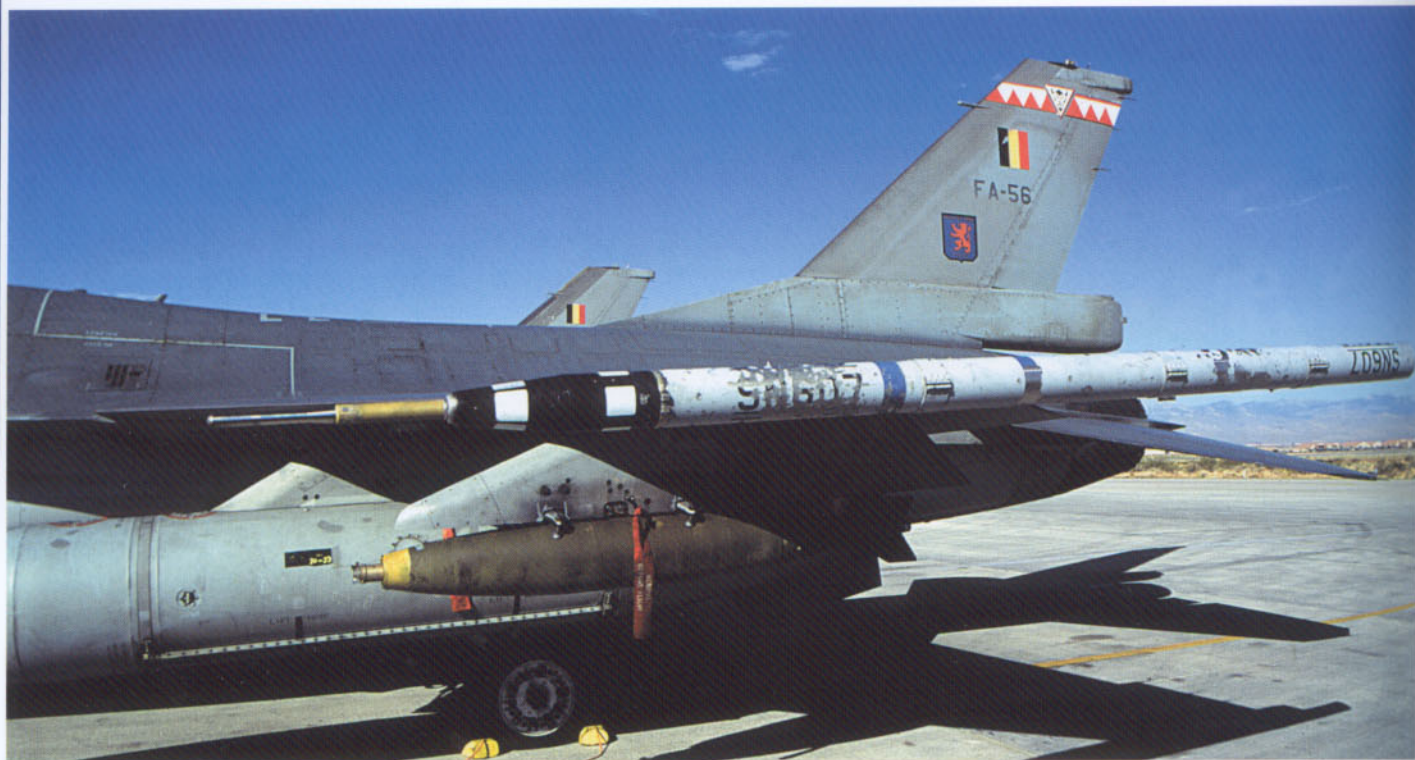
Photos above and below: F-16s carrying an ACMI pod. This is an airborne air data sensor, electronic altimeter and inertia sensor; in this it can send data to ground receiving stations. It is also used in training Air Combat Maneuvering, to judge the effects of simulated weapons fire and provide data for debriefing the pilots performance.
