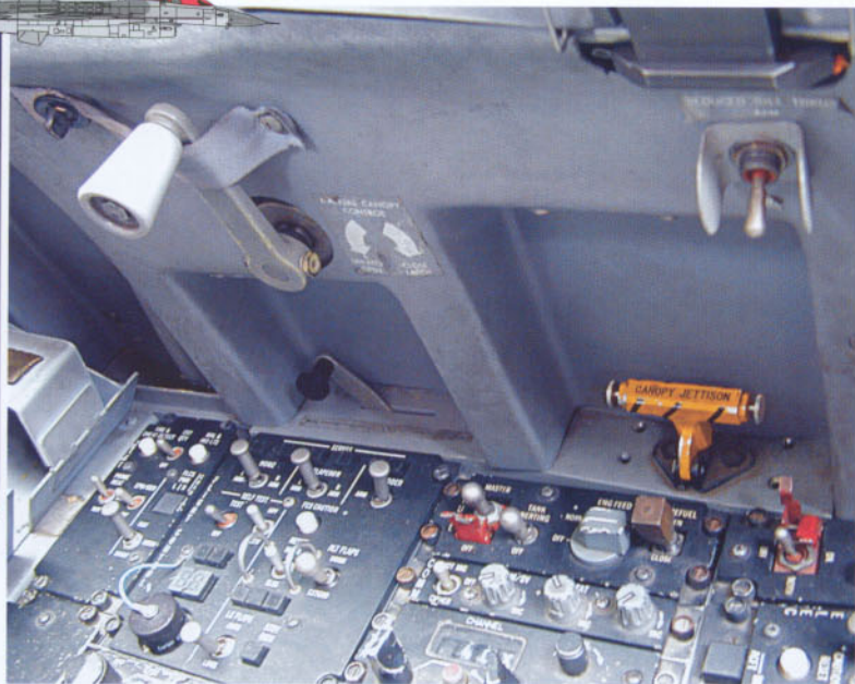
Above: When seated in the cockpit of the F-16 A and looking to the aft left side, this is what you see. The grey crank is to manually open the canopy in case of a power failure. The yellow handle in front, ejects the canopy and with the switch above it opens or closes the pilot the canopy.
