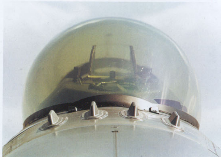
Below and right: Belgium, the Netherlands, Denmark, Norway and Portugal have updated most of their F-16s to MLU standards, and one of the new features are the Advanced IFF antennas just in front of the canopy.
