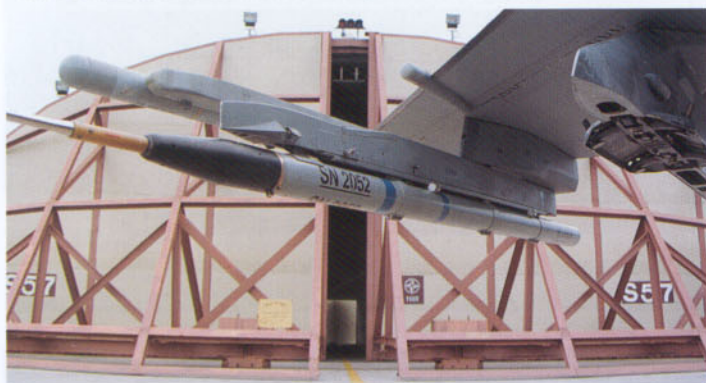
Below: The F-16 is stealthier than you might think, due to the Radar-reflecting paint applied. Ground radars have difficulties to interpret the right location of an F-16 on their screens, which can be dangerous for civilian aircraft. The AMA has a Radar Reflecting metal head mounted on the tube of the Sidewinder, and gives the right location of the F-16 during peace time. Normally it is always placed on Station 9, the right hand side wing tip station.
