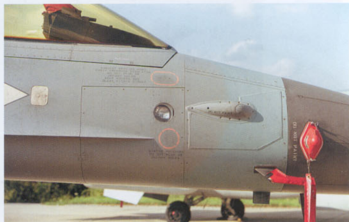
Above: This F-16C is in service with the Hellenic AF. It too has a searchlight, but this time it is installed on the right side of the aircraft and more aft located.
