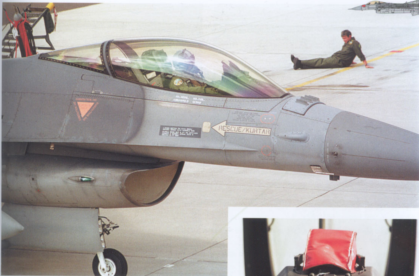
Above and right: an F-16C from Turkish Air Force. Note the four IFF antennas on the nose, which are of a different type than the ones of the European F-16A MLU.
