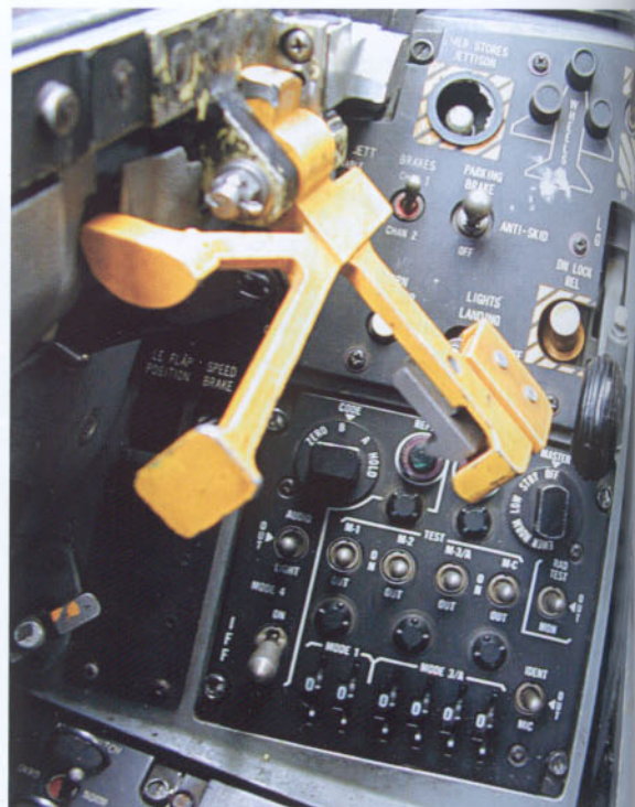
Above: When the pilot has closed the canopy, he pushes this yellow handle to the wall of the cockpit to lock and seal the canopy.
