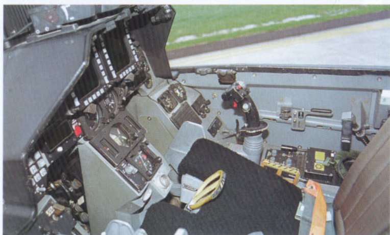
One difference between the single and the two seat F-16s, is the air conditioning grid. In the latter, do not have the box-shaped grids. Note the detail of the canopy framing in this photo.
