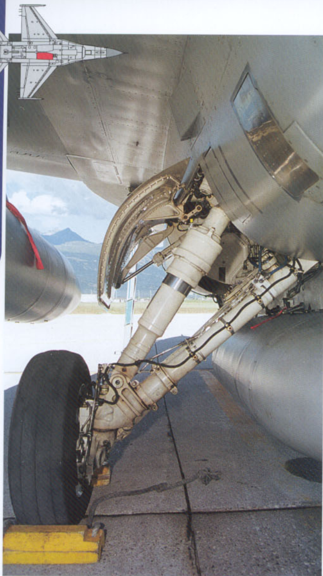
Above: The left main gear strut looking forward, with the hydraulic lines feeding the brakes nicely visible. Below: inside details of the main gear door of the A model (left) and C model (right). Note that the actuator that closes the door is removed on the left picture. A front view of this actuator is given on the opposite page.
