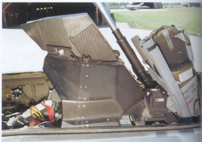
One difference between the single and the two seat F-16s, is the air conditioning grid. In the latter, do not have the box-shaped grids. Note the detail of the canopy framing in this photo.
