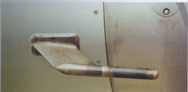
Above and below: the Air Data Probe, which can be found just after the radome. Note the tiny ECM-receiver in the photo above, a feature only to be found on the Belgian Air Force F-16s as part of the CARAPACE ECM system.
