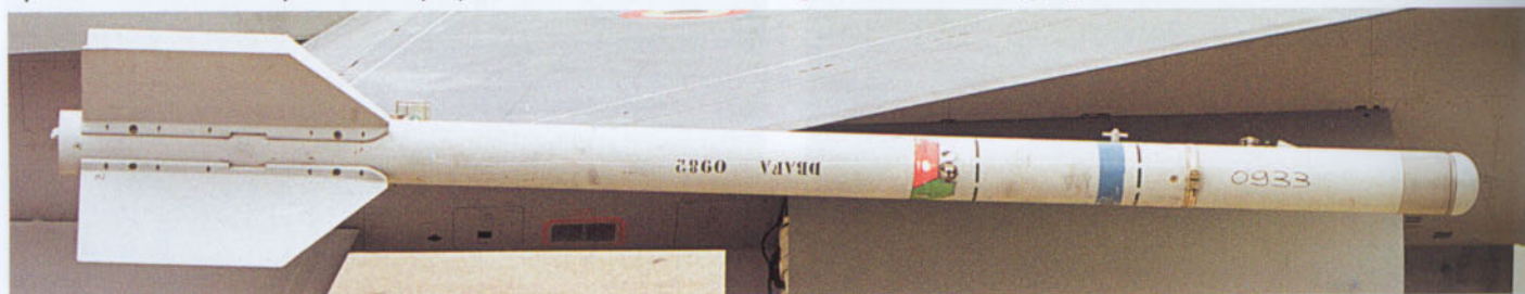
Below: The F-16 is stealthier than you might think, due to the Radar-reflecting paint applied. Ground radars have difficulties to interpret the right location of an F-16 on their screens, which can be dangerous for civilian aircraft. The AMA has a Radar Reflecting metal head mounted on the tube of the Sidewinder, and gives the right location of the F-16 during peace time. Normally it is always placed on Station 9, the right hand side wing tip station.
