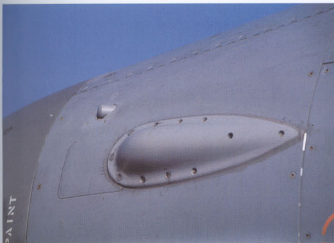
Above: The teardrop shaped fairing houses the Radar Homing and Warning Sensor (RHAW).
