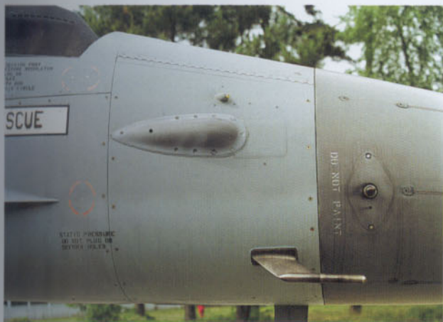
Above and below: the Air Data Probe, which can be found just after the radome. Note the tiny ECM-receiver in the photo above, a feature only to be found on the Belgian Air Force F-16s as part of the CARAPACE ECM system.
