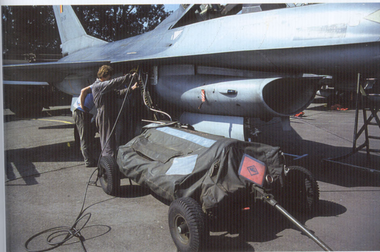
Loading and emptying the ammo drum feeding the M61 20mm Vulcan cannon is done at the starboard strake, right in front of the EPU exhaust.
