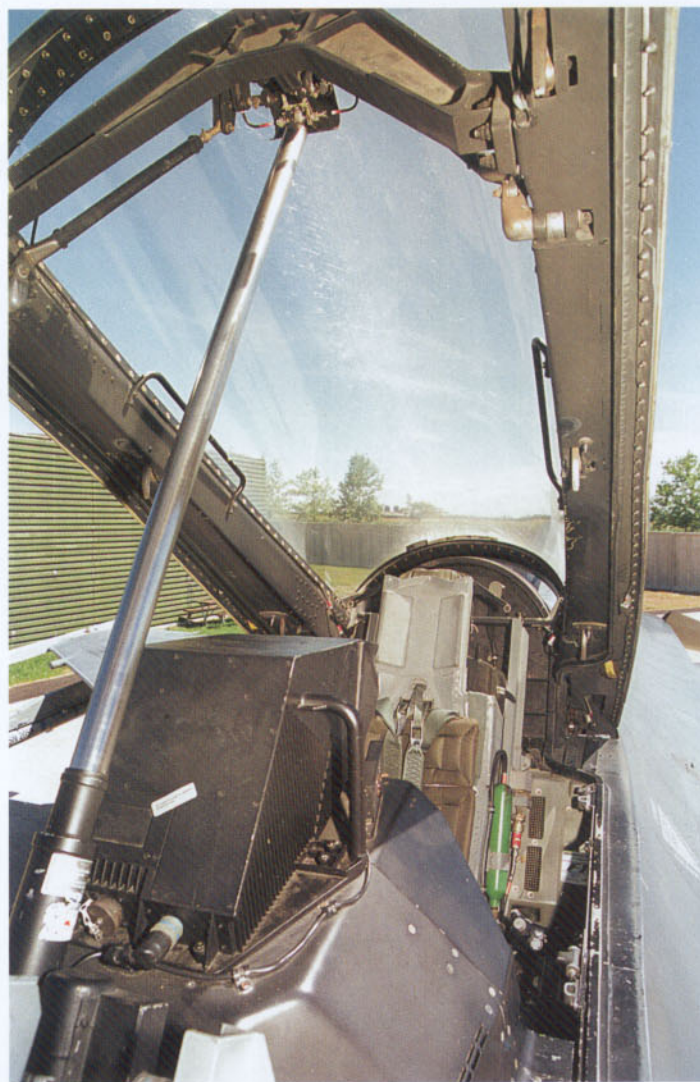
The Cockpit of F-16 D Block 40, 89-2178, flying with the Aviano Buzzards. Note the HUD Repeater in front of the backseat.
