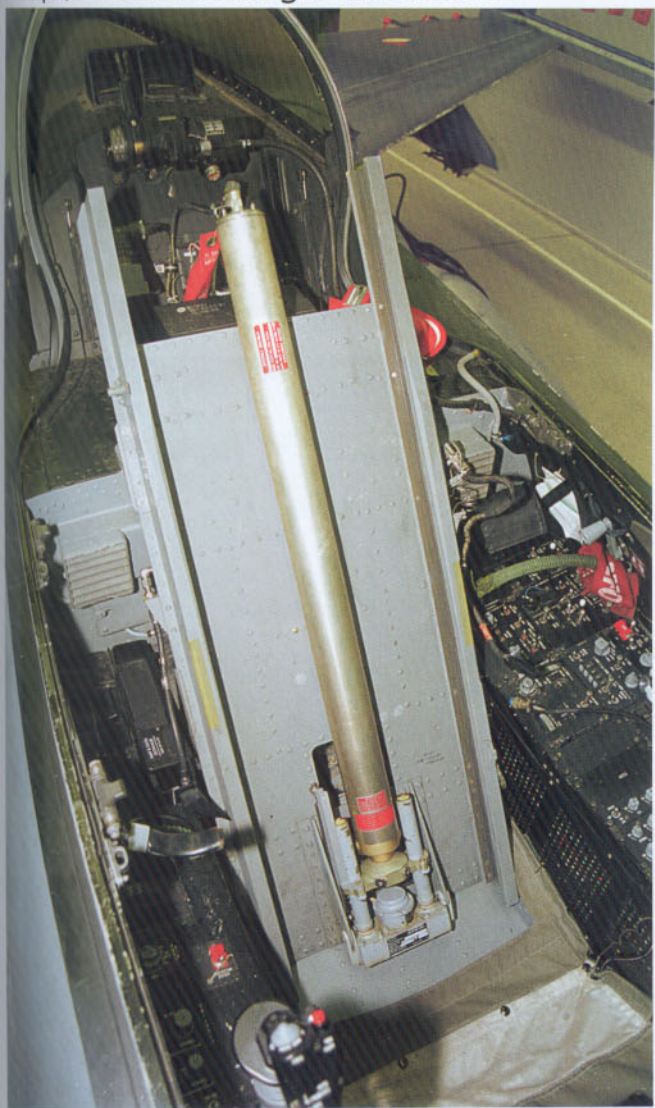
More details of the MLU-cockpit. Interesting to see is the partially black ejection seat. Notice the black walls of the cockpit, for the obvious night vision reasons.
