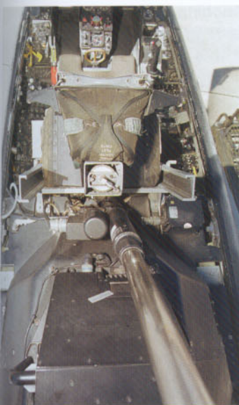
The Cockpit of F-16 D Block 40, 89-2178, flying with the Aviano Buzzards. Note the HUD Repeater in front of the backseat.
