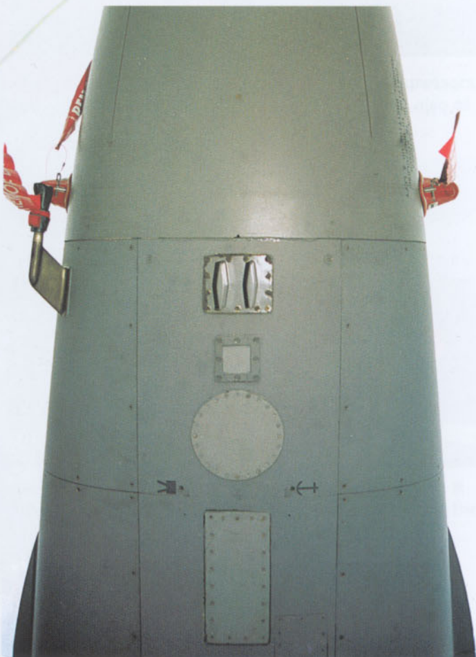
Above and below: the Air Data Probe, which can be found just after the radome. Note the tiny ECM-receiver in the photo above, a feature only to be found on the Belgian Air Force F-16s as part of the CARAPACE ECM system.
