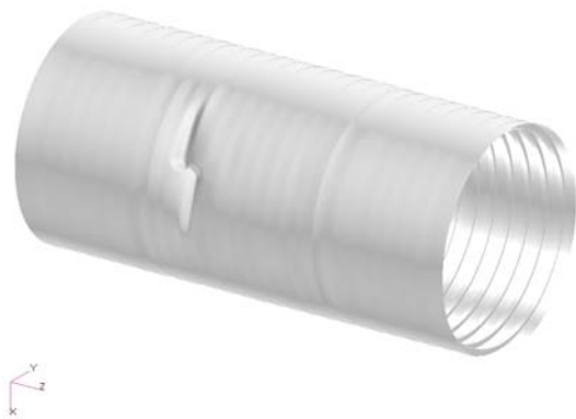
Figure 4 Interframe collapse in a model representative of a submarine compartment
