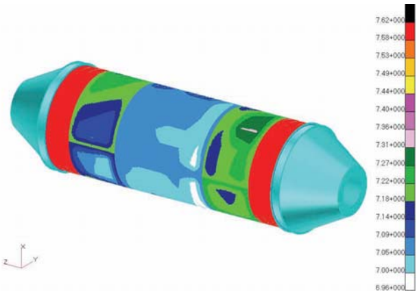
Figure 6 Plating thickness of additional 29-frame model.
