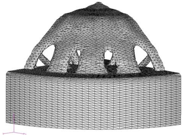
Figure 16: Solid mesh representation of topology optimised conceptual design solution, external perspective.
