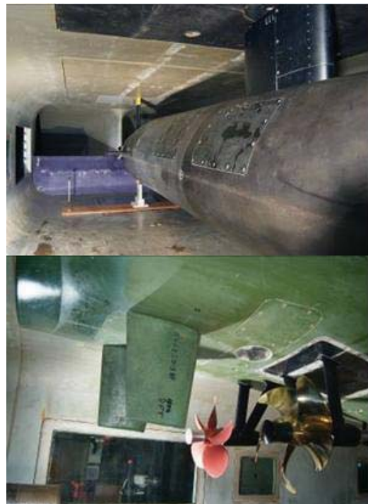
Figure 1: Model test arrangements for cavitation viewing in the QinetiQ Cavitation Tunnel
