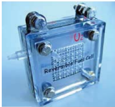
Figure 2: Horizon Fuel-Cell Technologies 0.6W reversible fuel-cell [7].
