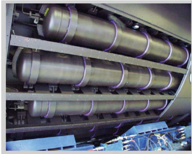
Figure 1: U212/4 class metal hydride cylinders [6].
