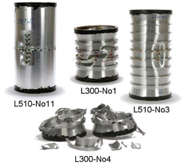
Figure 2: Typical undamaged and corroded cylinders
