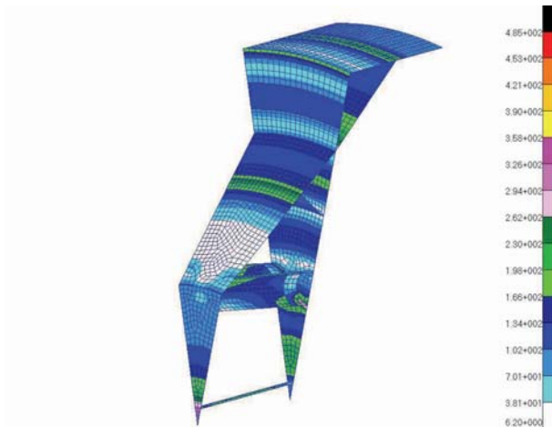
Figure 18: von Mises stresses in 10 m size optimised conceptual solution under 7 MPa load.
