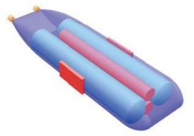
Figure 6: Alternative concept trading weapons capability for endurance with conventional lithium-ion batteries
