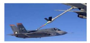
**Figure 4:** Manually flown aircraft refueling boom. (Lockheed-Martin Tactical Aircraft Systems photo.)
