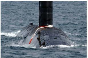
Figure 7 – Photograph of the Fin Harness rigged by the submarine crew
