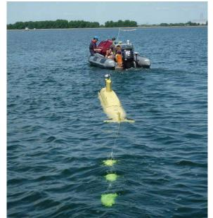
Figure 8 – Photograph of an open water tow trial on a Resolution Class submarine model with drogues at the stern to keep it on the towed course
