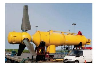
Figure 9: 500 kW demonstrator tidal generating system operating at European Marine Energy Centre in Orkney since September 2010 (Rolls-Royce Tidal Generation Ltd)
