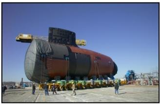
Changes to the Manufacturing Assembly Plan (MAP) Facilitate a Four Module Concept
