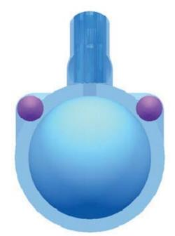
Figure 15: Bow view of Design V3 showing UUV stowages in upper casing
