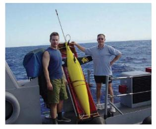
Figure 3. University of Washington's Seaglider in its handling cradle [23]
