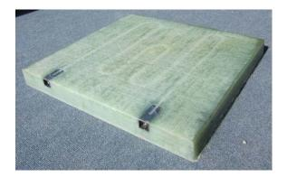
Figure 7: CSV Flat Panel with Optical Fibre Strain Sensors (Insensys)
