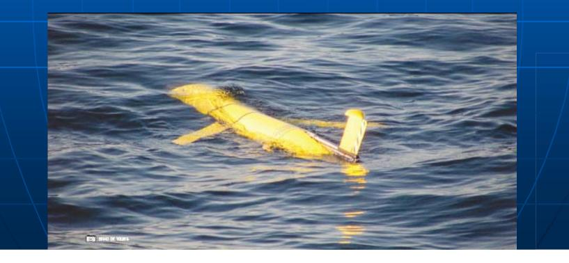
Underwater Gliders have proven utility in oceanography and are capable of flights measured in weeks and hundreds of miles
