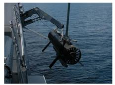
Figure 2 – Lockheed Martin Semi-Submersible Remote Minehunting System [5]
