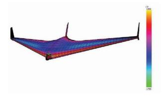
Figure 8. Distribution of pressure coefficient on X-Ray Glider computed by inviscid panel CFD software USAERO/OMNI3D [29]
