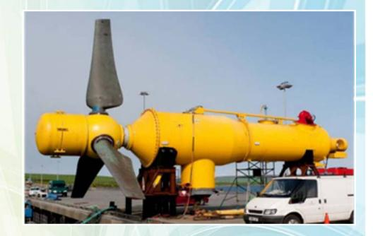
Figure 9 500 kW Demonstrator Tidal Energy System Operating at European Marine Energy Centre in Orkney
