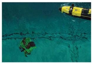
Figure 1 – Photograph of a parachute sea anchor on test with a submarine model
