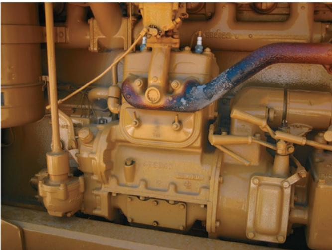
**FIGURE 7-1** A pup engine starter motor.
