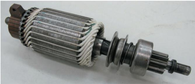
**FIGURE 7-11** A typical armature and how the loops of wire are embedded into the core.
