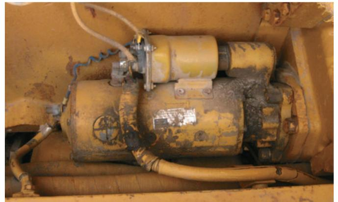
**FIGURE 7-2** A typical arrangement of a heavy-duty electric starter on a diesel engine.
