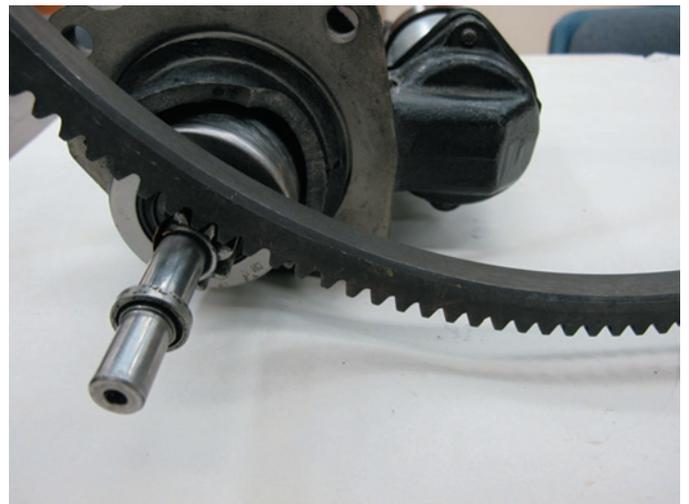
**FIGURE 7-3** A starter assembly engaging with a flywheel ring gear.
