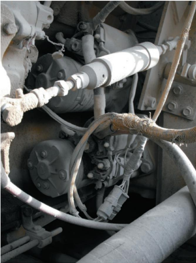
**FIGURE 7-4** A double starter assembly arrangement.
