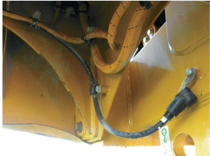
**FIGURE 7-21** A properly secured battery cable.
