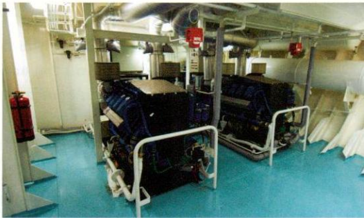
▲ Two diesel generator sets on board a container-feeder with a Scania diesel engines.
