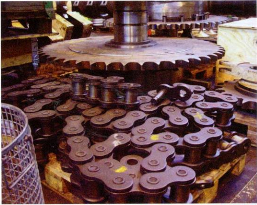
▲ A chain and a gearwheel for driving the camshaft for a large two-stroke crosshead engine of MAN-B&W.
