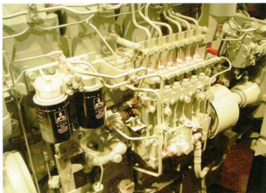
▲ A block fuel pump with six independent high-pressure in-line plunger pumps.
