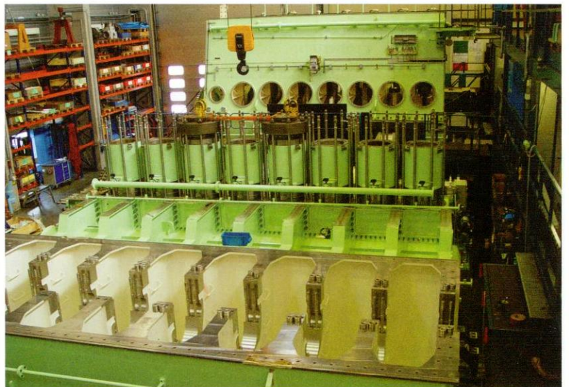
▲ The manufacture of two-stroke crosshead engines at MAN-B&W, Frederikshavn, Denmark.
