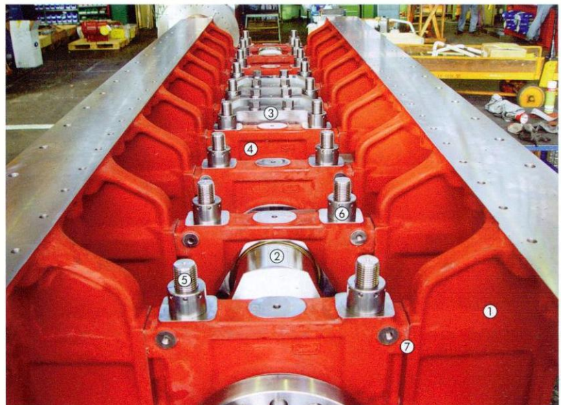
▼ A block in an in-line engine rotated 180° for the mounting of the underslung crankshaft.
