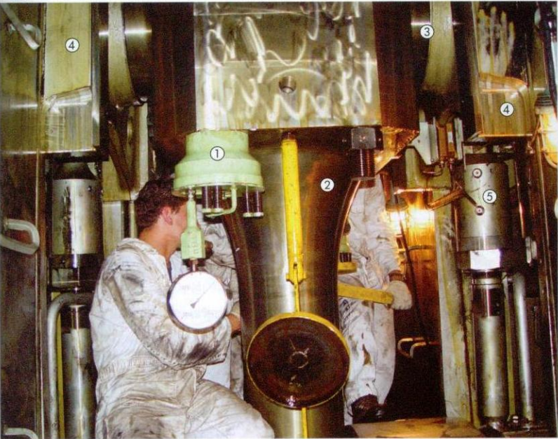
Maintenance on the crosshead. Fitting hydraulic jackets to the studs for attachment of the connecting rod to the crosshead.
