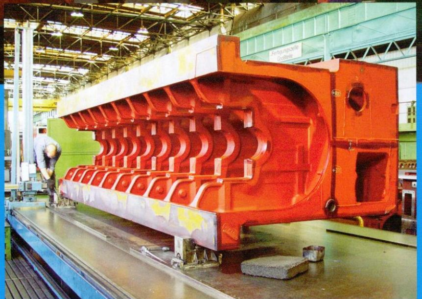
A cast engine block aligned for the initial machining process.
