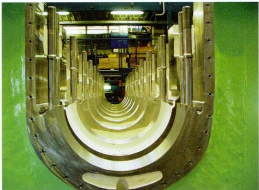
▲ The welded steel crankshaft bed of a crosshead engine; it is of utmost importance that the crankshaft is placed in line.
