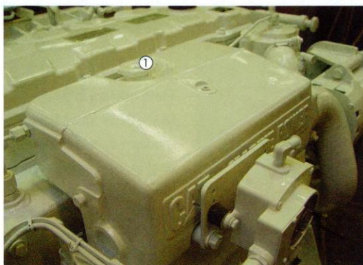
► A coolant storage expansion tank in a small high-speed four-stroke diesel engine.
