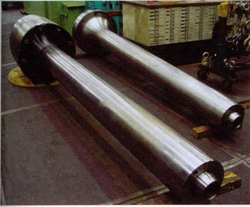
▲ A piston with piston rod and a bare piston rod after repair.
