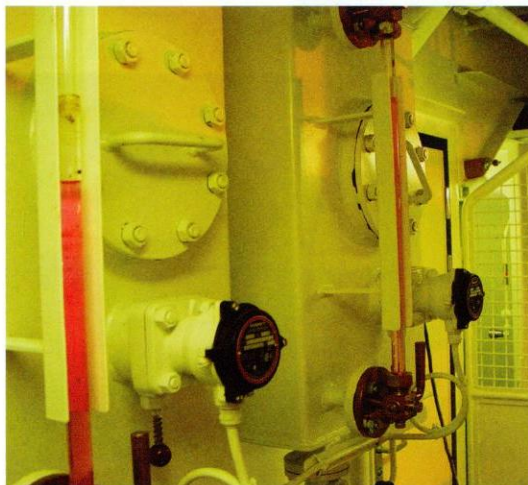
◀ Two fresh-water expansion tanks for high-speed four-stroke Deutz-diesel engines.
