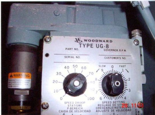
Detail of the UG-3 Woodward governor with the ‘Speed droop’ and ‘Speed Setting’ settings.
