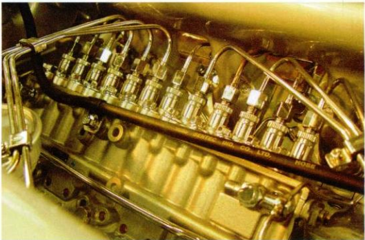
A block fuel pump for a twelve cylinder four stroke high speed V-diesel engine.
