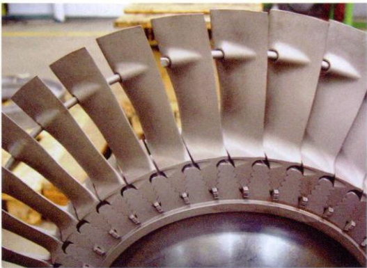
▲ The shaft and the blades in the exhaust-gas turbine of the turbo blower are manufactured from high-alloyed steel for resistance to high temperatures and corrosion caused by chemicals.
