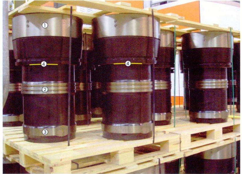
▲ The cylinder liner of a modern highly loaded diesel engine.
