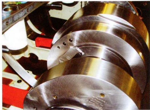
▲ A section of the camshaft for a low-speed two-stroke-crosshead engine, manufacturer Wärtsilä, type RTA 96 C.
