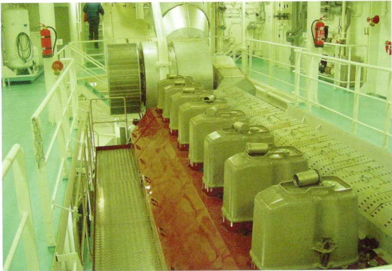
▲ A medium-speed four-stroke in-line engine used for propulsion in a 'feeder-container ship'.
