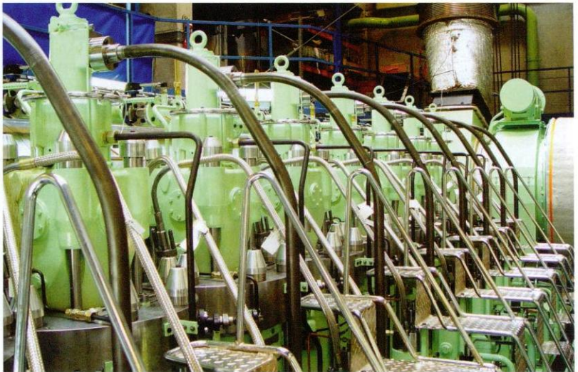
▲ The cylinder head of a crosshead engine with in the background the turbo blower.
