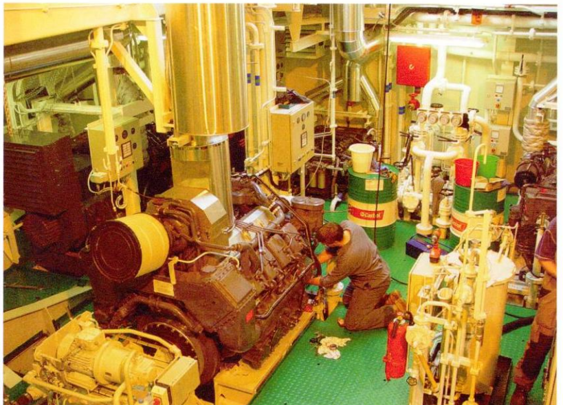
▼ A Deutz propulsion engine with reduction drive to the controllable pitch propeller on a dredger of the Iran government.
