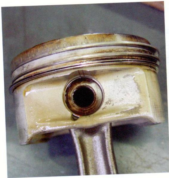
▲ A piston for a small engine with two compression rings and one oil-scraping ring.
