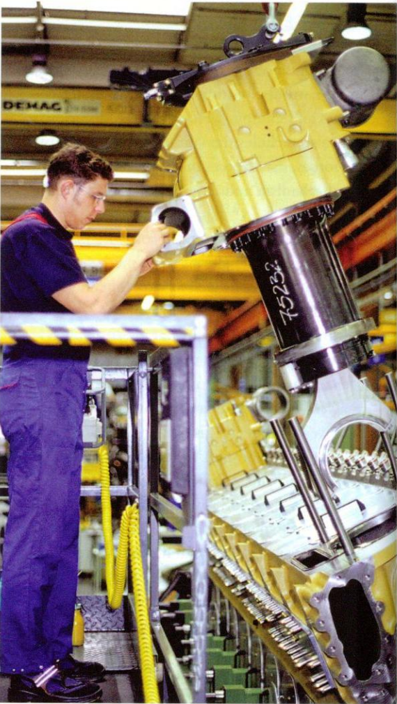
▲ Mounting the complete cylinder unit with cylinder head, piston, connecting rod and cylinder liner in an eighteen-cylinder MTU V engine block, type 8000, category II in Friedrichshafen, Germany.
