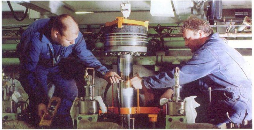
▲ Disassembling a piston with piston rod.
