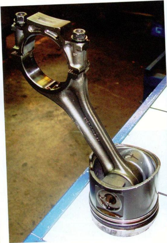
▼ An aluminium piston for an engine category I or II.
