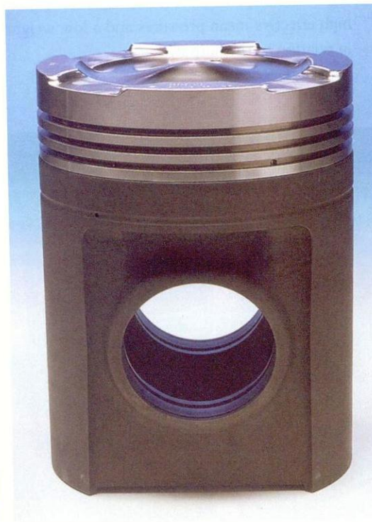
◀ A piston with a cast steel piston crown and cast iron piston skirt.
