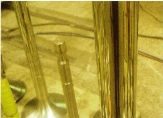
▲ A chromed valve stem that is very wear-resistant and resistant to chemical corrosion.
