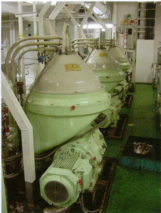
▲ Heavy oil separators in the machine room of a large container ship.
