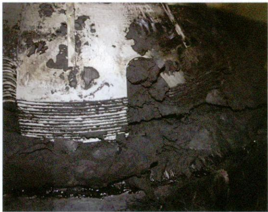
▶ A completely soiled disc stack package in a heavy oil separator.
