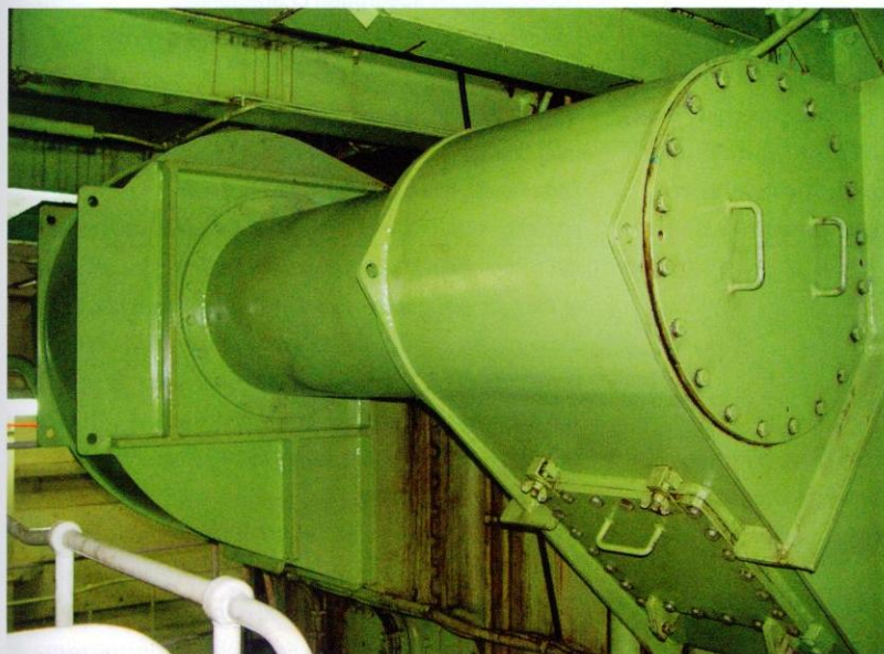
◀ The electrically driven auxiliary blower in a two-stroke crosshead engine.
