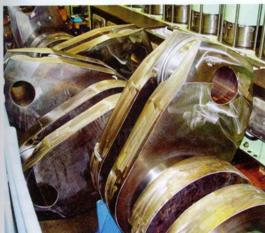
▲ A partially built crankshaft for a low-speed two-stroke crosshead engine of MAN-B&W, type MC 50.
