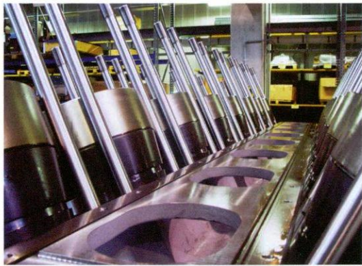
▲ The engine block of a V-engine with fitted cylinder liner and cylinder head bolts. In the middle the air inlet manifold.
