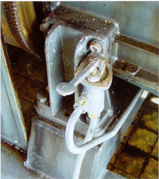
▲ A manual air stop valve for a starting-air turbine/motor on a older Kromhout diesel engine – Category I.
