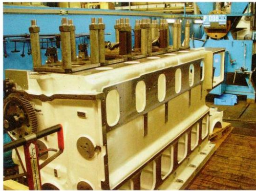
◀ A cast block of an in-line engine in manufacture.
