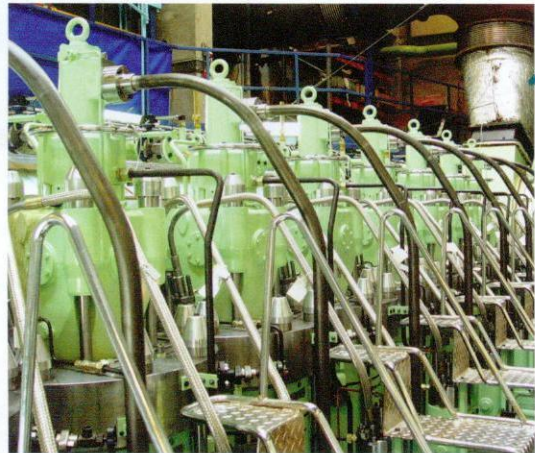
▲ Cylinder heads with on top the hydraulically driven exhaust valves of a MAN-B&W two-stroke crosshead engine and a cylinder bore of 500 millimetres.
