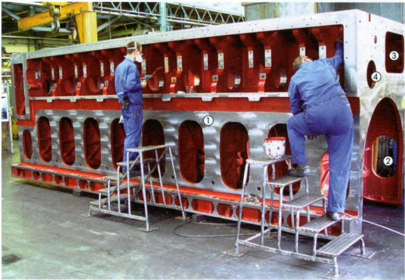
▲ The cylinder block of a Caterpillar Mak 43 in-line engine. 1 engine block 2 position of crank shaft 3 scavenge air space 4 position cam shaft The air supply to the cylinders is integrated into the solid block. Here only the crank shaft bearing caps have been fitted.
