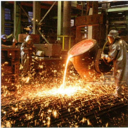
▲ The casting of a large block for a four-stroke diesel engine.
