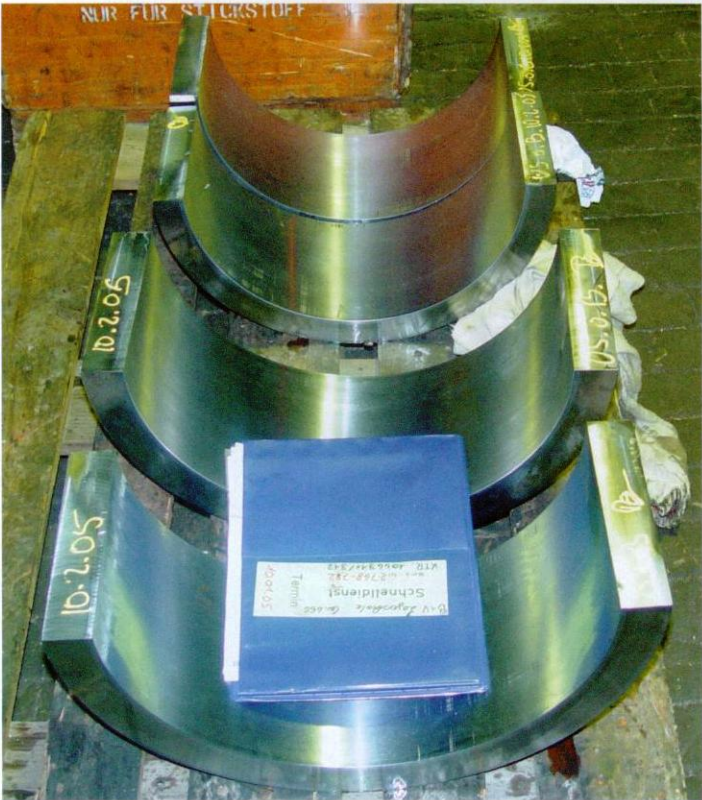
White-metal bearing shells for a two-stroke crosshead engine by MAN-B&W.
