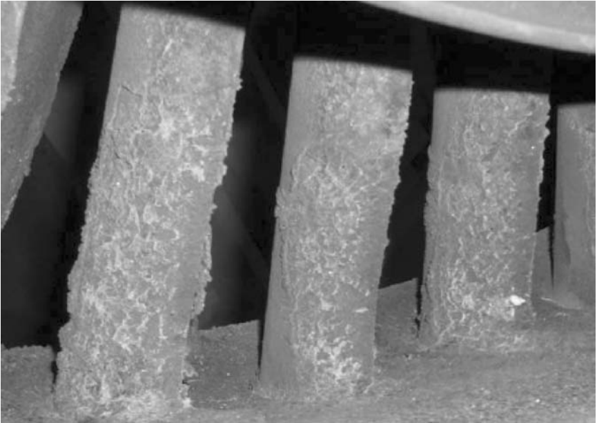
Figure 22-30. Bowed turbine nozzle vanes.
