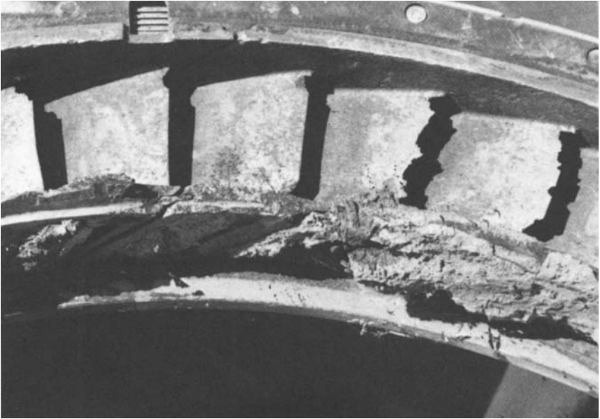
Figure 22-29. Burnt first-stage nozzle.
