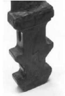
Figure 22-44. Erosion and corrosion in the blade fir tree region.
