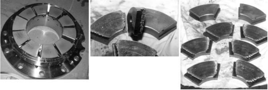
Figure 22-51. A failed thrust bearing.
