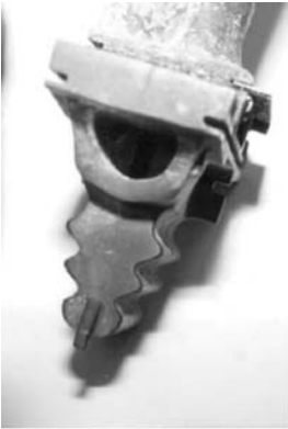
Figure 22-44. Erosion and corrosion in the blade fir tree region.
