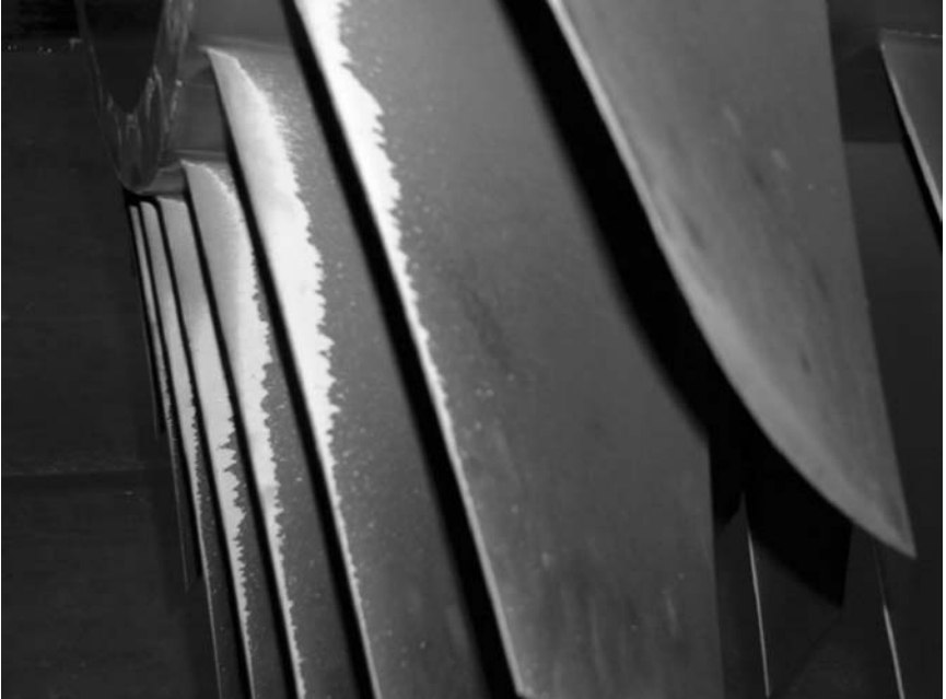
Figure 22-5. Coating erosion found at the leading edge of the first stages of the compressor.
