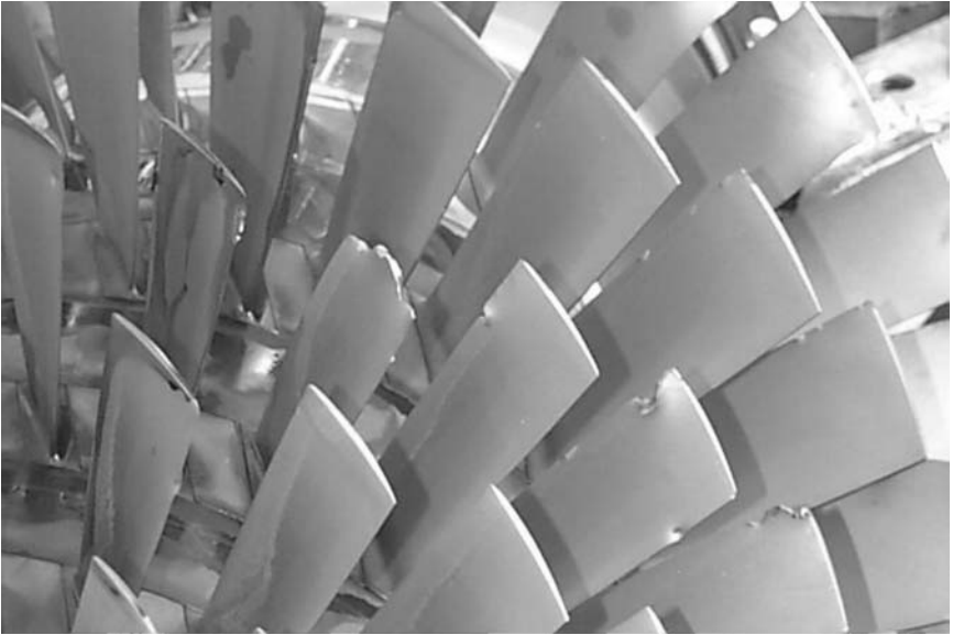
Figure 22-17. Damaged blades due to domestic object damage (DOD).
