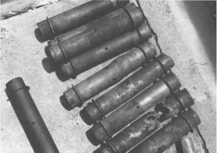
Figure 22-19. Damaged cross-over tubes.
