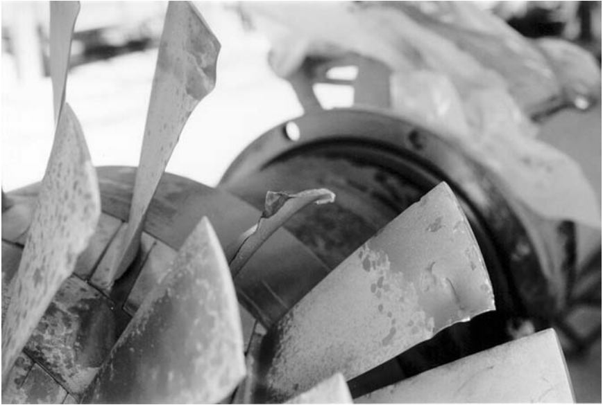
Figure 22-12. Failure of the first-stage compressor.
