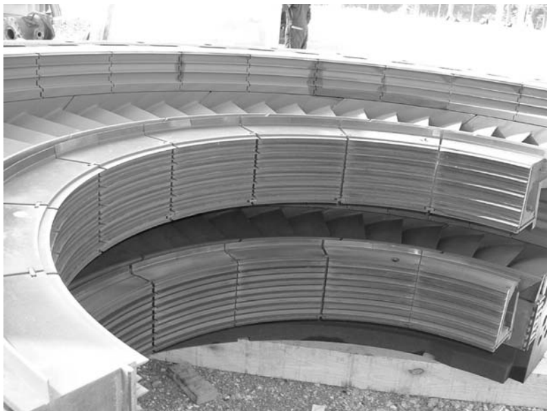
Figure 22-42. Turbine casing and vane sections with labyrinth seals.
