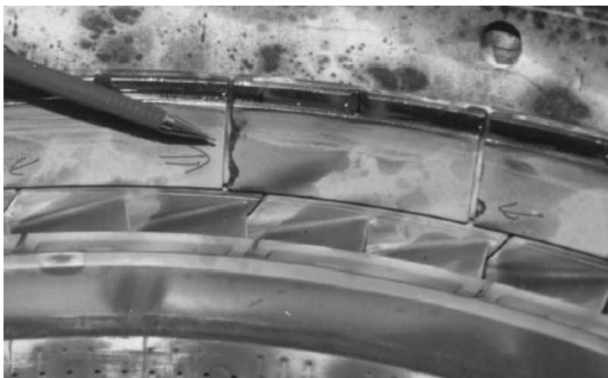
Figure 22-43. First-stage shroud ring heavily burnt.
