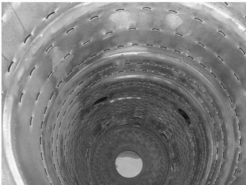
Figure 22-22. Can-annular combustor used in a crude oil application.
