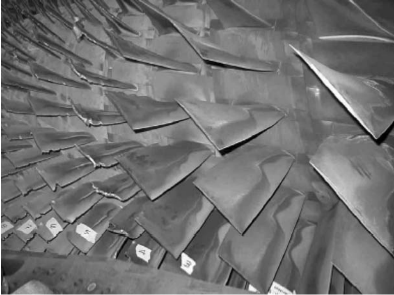
Figure 22-11. Compressor blade damage due to domestic object damage (DOD).
