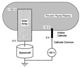
Fig. 8-17. A large area of high voltage solar array exposed to the thruster plume causes the cathode common to float the order of the array voltage positive of spacecraft chassis ground.
