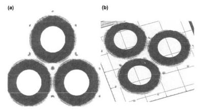
Fig. 5-26. CEX-3D calculation of the pits-and-grooves erosion wear patterns that match the experimental patterns shown in (a) Fig. 5-22(a) and (b) 5-22(b).
