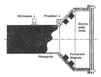
Fig. 4-39. Schematic of the MUSES-C 10-cm microwave source showing the strong magnets and small volume characteristic of these thrusters (from [54]).
