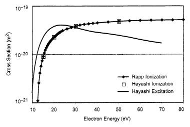
Fig. 4-15. Ionization and excitation cross sections for xenon [28,29].
