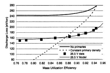
Fig. 4-20. Discharge loss predictions for the cases of no primary electron density and a constant primary electron density showing the poor agreement with the measurements.
