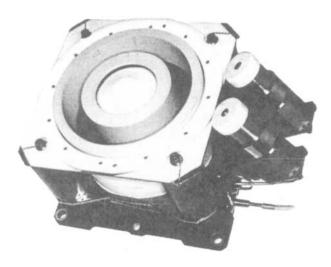
Fig. 9-9. Photograph of an SPT-100 Hall thruster (from [33]).
