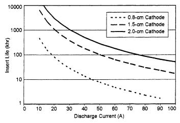
Fig. 6-47. Calculated lifetime in thousands of hours versus the discharge current for three different LaB<sub>6</sub> cathode diameters.
