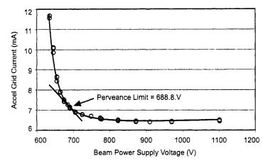
Fig. 5-8. Accel grid current versus the screen supply voltage for the NSTAR thruster at TH15 parameters, showing the perveance limit.
