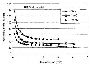
Fig. 5-18. Threshold electric field for pyrolytic graphite with grid apertures (from [36]).
