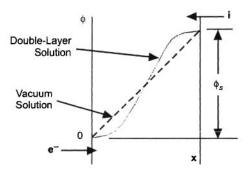
Fig. 3-5. Schematic of the double-layer potential distribution.
