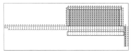
Fig. 6-26. Hollow cathode thermal model input geometry with the different types of cells numbered and the boundary conditions indicated by numbers. Negative numbers indicate radiative boundaries [30].
