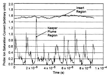
Fig. 6-57. Ion saturation current oscillations inside and outside the cathode, showing oscillation location.
