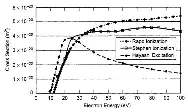
Fig. D-1. lonization and excitation cross sections for xenon.
