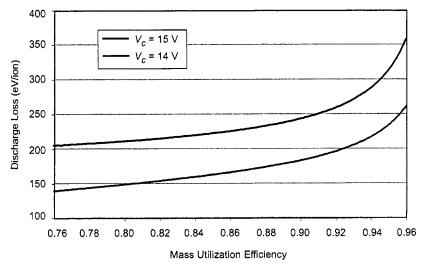
Fig. 4-27. Discharge loss calculated for Kaufman thruster example.
