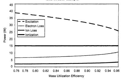
Fig. 4-7. Discharge loss for each of the energy loss mechanisms for the ideal thruster with reduced anode area.
