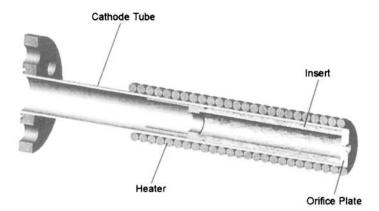
Fig. 6-1. Typical hollow cathode geometry of a refractory metal tube with an emissive insert inside and a heater wrapped on the outside.
