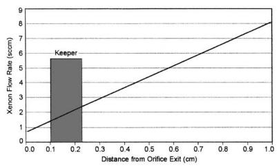
Fig. 6-34. Flow rate at which the Langmuir ratio is equal to one and double layers can be formed as a function of the distance downstream from the NEXIS cathode orifice [39].
