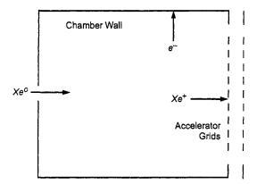
Fig. 4-3. Idealized ion thruster with the ions assumed going to the grids and electrons going to the chamber wall.
