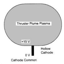
Fig. 8-15. The thruster neutralizer hollow cathode generates a plasma typically 10 to 20 V above the cathode common.
