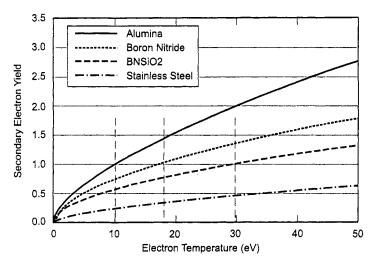
Fig, 7-11. Secondary electron yield from the power-curve fits versus electron temperature, showing the cross-over value at which the yield equals one.
