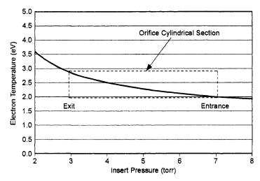
Fig. 6-17. Orifice electron temperature calculated from the 0-D model through the orifice for the NSTAR discharge cathode at TH15.
