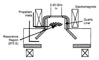
Fig. 4-36. Schematic of microwave ion source with a volumeresonance zone of strong magnetic field produced by electromagnets.
