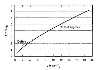
Fig. 3-4. Normalized sheath thickness as a function of the normalized sheath potential showing the transition to a Child-Langmuir sheath as the potential becomes large compared to the electron temperature.
