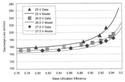
Fig. 4-18. Example of the discharge loss versus mass utilization efficiency for three discharge voltages in the NEXIS thruster [38].
