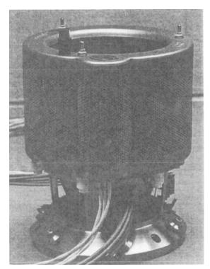
Fig. 9-5. Photograph of the T5 Kaufman ion thruster (photo courtesy of Qinetiq, Limited).
