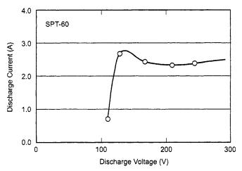
Fig. 7-17. Current versus voltage for one operating condition in the SPT-60 ([redrawn from [4]), showing the non-monotonic current variations usually observed in Hall thrusters at low discharge voltages.
