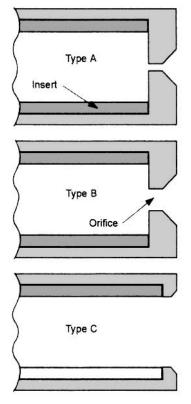
Fig. 6-5. Schematics of the three characteristic types of hollow cathodes (A, B, and C) depending on the orifice geometry.
