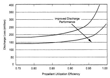
Fig. 2-3. Ion thruster performance curves consisting of discharge loss versus propellant utilization efficiency.
