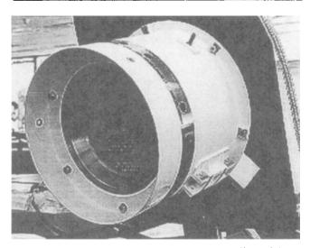
Fig. 9-6. Photograph of the RIT-10 rf ion thruster (from [16]).
