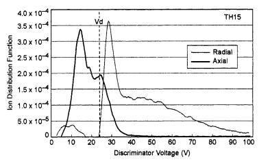
Fig. 6-51. Ion energy distribution measured on axis and radially away from an NSTAR hollow cathode (from [46]).
