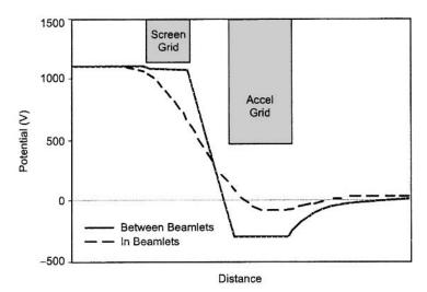
Fig. 5-9. Potentials on-axis in an individual beamlet and between the beamlets intersecting the grids.
