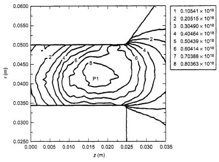
Fig. 7-15. Average plasma density computed by HPHall for the SPT-100, with the peak plasma density at P1 =  $8 \times 10^{17}$  m<sup>-3</sup> (from [30]).
