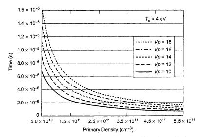
Fig. F-3. Spltzer's slowing-down time as a function of the plasma density with an electron temperature of 4 eV for several primary energies.
