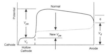
Fig. 4-22. Transition of the plasma potential to negative relative to the anode due to an anode area decrease, which results in a lower primary electron energy.
