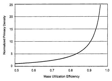
Fig. 4-17. Normalized primary electron density as a function of mass utilization efficiency.
