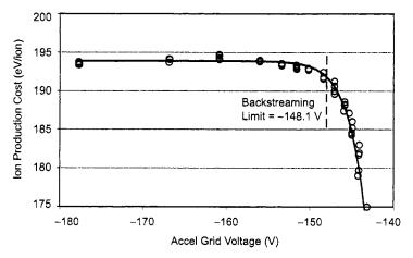
Fig. 5-12. Ion production cost for NSTAR TH15 versus applied accel grid voltage, showing the onset of electron backstreaming as the voltage is decreased.
