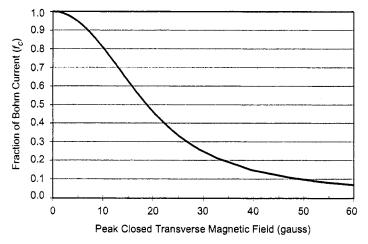
Fig. 4-14. Fraction of the Bohm current density to the anode wall as a function of the transverse magnetic field strength for the NSTAR ion thruster [13].
