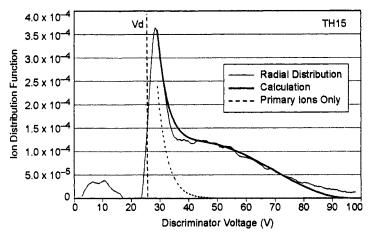
Fig. 6-53. The xenon ions gain most of their kinetic energy in the sheath and the potential well on axis (from [65]).
