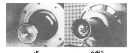
Fig. 6-50. NSTAR discharge cathode before and after the ELT wear test, showing complete sputter erosion of the keeper electrode [38].
