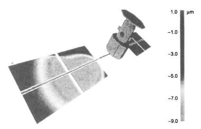
Fig. 8-14. Contours of the erosion (negative numbers) and deposition depths (positive numbers) due to sputtering during operation of the SPT-100 Hall thruster onboard the Express-A spacecraft. The calculation was performed with EPIC [6].
