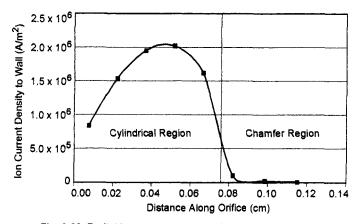
Fig. 6-22. Radial ion current to the orifice wall as a function of distance along the axis in the NSTAR neutralizer cathode at TH15.
