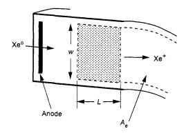
Fig. 7-5. Schematic cross section of the plasma in the Hall thruster channel.
