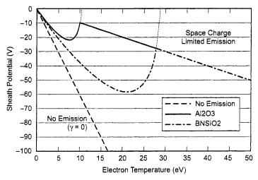
Fig. 7-13. Sheath potential versus electron temperature for two materials. The sheath transitions to space-charge limited where the dashed lines intersect the potential curves.
