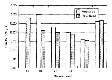
Fig. 8-4. Calculated and measured charge-exchange ion fluxes in the plume of NSTAR at various operating points (from [8]).
