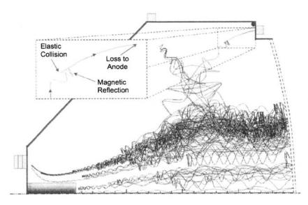
Fig. 4-43. Example primary electron trajectory calculated inside the NSTAR discharge chamber (from [60]).
