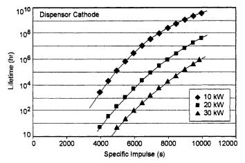
Fig. 6-46. Model prediction of NEXIS dispenser cathode life versus lsp for several thruster powers [47].
