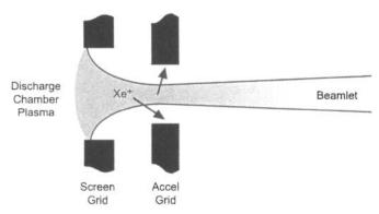
Fig. 5-20. Ions that cause barrel erosion are generated by charge exchange upstream and within the accelerator grid aperture.
