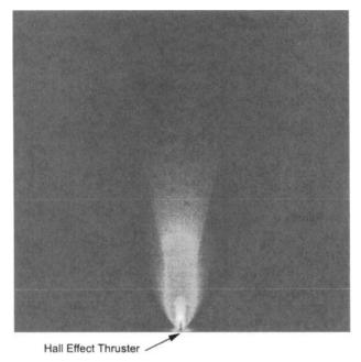
Fig. 8-2. Total ion density in the plume of a 4-kW Hall thruster.
