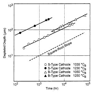
Fig. 6-44. Depletion depth of a porous tungsten insert as a function of time for cathodes at different temperatures (redrawn from [51]).
