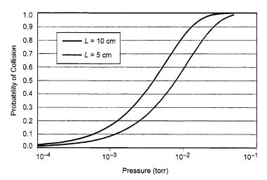
Fig. 4-35. Probability of an electron-neutral collision before leaving the resonance zone length indicated as a function of neutral pressure for 2-eV electrons.
