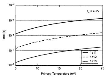
Fig. F-2. Spitzer's slowing-down time as a function of the primary electron energy for three densities of electrons at 4 eV.
