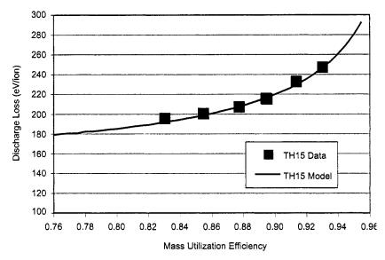
Fig. 4-19. Discharge loss versus mass utilization efficiency for the NSTAR thruster at the high power TH15 throttle point.
