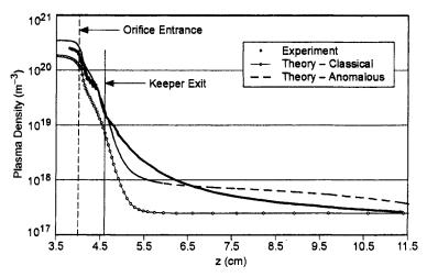
Fig. 6-35. Plasma density profile on axis for the NEXIS cathode showing that an anomalous resistivity is required to provide sufficient ionization to come close to matching the experimental data [41].
