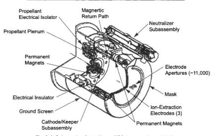
Fig. 9-1. Schematic of the 13-cm XIPS thruster (from [4,10]).
