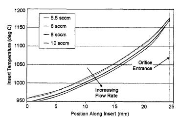
Fig. 6-42. Insert temperature profile for an SSC hollow cathode operating at 12 A of current for several different gas flow rates (redrawn from [50]).
