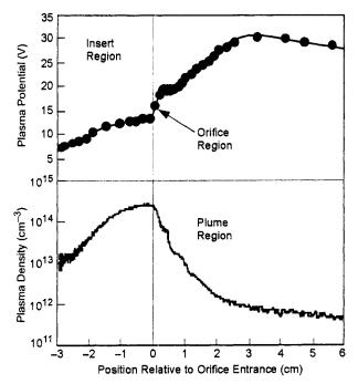
Fig. 6-3. Plasma potential (top) and density (bottom) measured on axis in the NEXIS hollow cathode at 25 A of discharge current.
