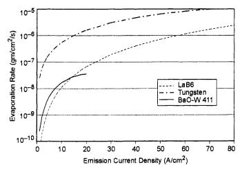
Fig. 6-8. Evaporation rate of Type-S 4:1:1-dispenser cathodes, LaB<sub>6</sub> and tungsten.
