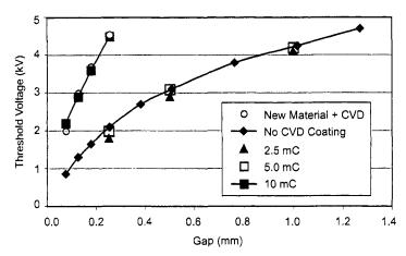
Fig. 5-16. Threshold voltage for carbon-carbon composite material after 10 arcs at various coulomb transfers (from [36]).
