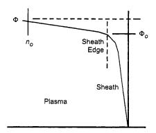
Fig. 3-3. Plasma in contact with a boundary.
