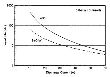
Fig. 6-48. Comparison of the calculated cathode lifetime versus the discharge current for the 0.8-cm outside diameter LaB6 cathode and the NSTAR dispenser cathode.
