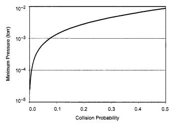
Fig. 4-30. Minimum pressure for starting a xenon rf thruster with a 5-cm interaction zone as a function of the probability of an electron having a collision.
