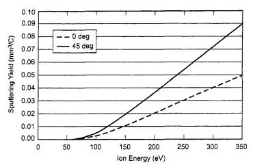
Fig. 7-21. Sputtering yield calculated for singly ionized xenon on BNSiO₂ versus ion energy for two incidence angles.
