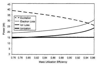
Fig. 4-6. Discharge loss for each of the energy loss mechanisms for the ideal thruster example.
