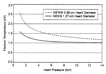
Fig. 6-9. Electron temperature in the insert region as a function of internal pressure for two cathode insert inner diameters.
