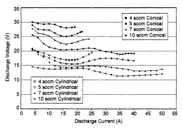
Fig. 6-54. Discharge voltage versus current for several hollow cathode flow rates for two anode configurations.
