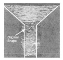
Fig. 6-24. Neutralizer cathode orifice cross section showing the erosion pattern after the NSTAR 30,152-hour extended life test [38].
