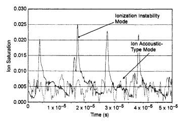
Fig. 6-56. Discharge voltage oscillations showing plasma plume mode oscillations with frequencies in >100-kHz range and ionization-related oscillations in the <100-kHz range.
