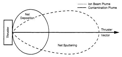
Fig. 8-13. Sputtering by main beam ions dominates at angles close to the thrust vector direction; deposition of thruster erosion products occurs at angles far from the thrust direction.
