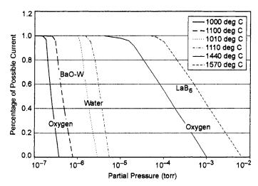
Fig. 6-49. Percentage of possible thermionic emission versus partial pressure of oxygen and water, showing the sensitivity of dispenser cathodes relative to LaB<sub>6</sub> (from [18]).
