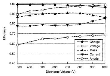
Fig. 7-9. Optimized anode efficiency and the individual efficiency terms versus discharge voltage for the NASA-173Mv2 Hall thruster operating at 10 mg/s (from [10]).
