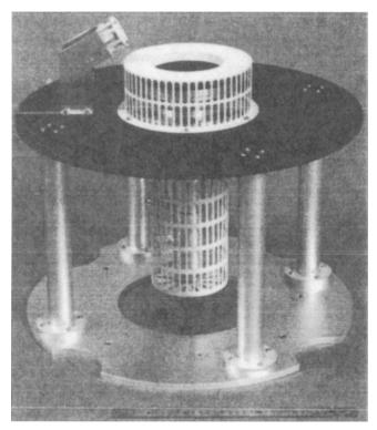
Fig. 9-7. Photograph of the µ10-ECR microwave discharge ion thruster (10-cm grid diameter) and microwave neutralizer [20].
