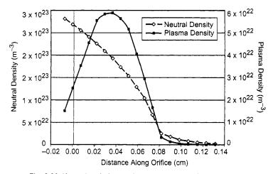
Fig. 6-20. Neutral and plasma densities calculated in the NSTAR neutralizer cathode orifice at the TH15 operation point.
