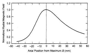
Fig. 7-4. Axial variation centerline radial magnetic field normalized to the peak radial field in the NASA-173Mv Hall thruster (from [11]).
