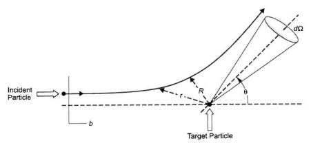
Fig. 8-20. Classic scattering diagram for an incident particle on a target particle.
