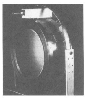
Fig. 9-3. Photograph of the NASA NSTAR ion thruster (photo courtesy of L-3 Communications, Electron Technologies, Inc.).
