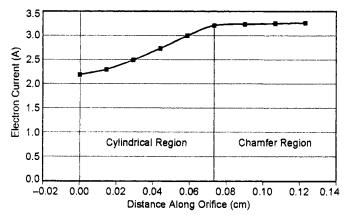
Fig. 6-21. Electron current as a function of distance along the axis in the NSTAR neutralizer cathode orifice at TH15.
