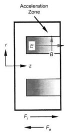
Fig. 2-2. Cross section of a Hall thruster showing electric and magnetic fields.
