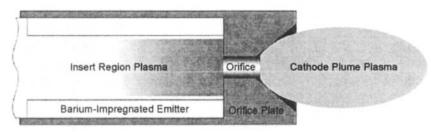
Fig. 6-2. The three plasma regions in a hollow cathode.
