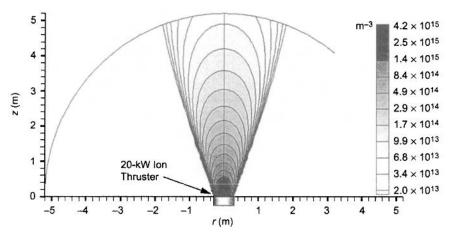
Fig. 8-9. Calculated primary ion beam density profile for the 20-kW NEXIS ion thruster [14].
