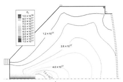
Fig. 4-47. Ion plasma density (m<sup>-3</sup>) for the NSTAR at throttle level TH15 [60].
