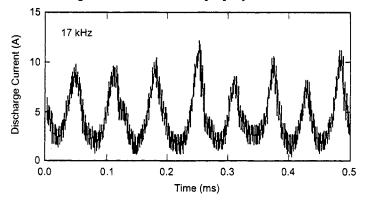
Fig. 7-18. Measured evolution of the discharge current for the SPT-100 (from [55]).
