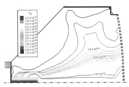
Fig. 4-44. Primary electron density (m<sup>-3</sup>) for NSTAR throttle level TH15 [60].
