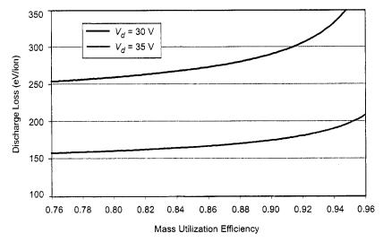
Fig. 4-28. Discharge loss calculated for Kaufman thruster example at two discharge voltages.
