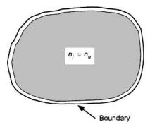
Fig. 3-2. Generic quasi-neutral plasma enclosed in a boundary.
