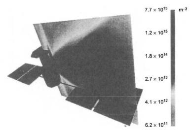
Fig. 8-5. EPIC model of the Express-A spacecraft showing the plume ion density profile during operation of the RT4 SPT-100 thruster (from [5]).
