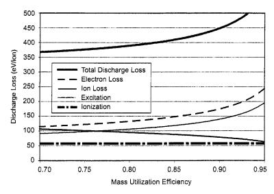
Fig. 4-32. Discharge loss calculated for the example rf ion thruster and the contribution from the four energy loss mechanisms.
