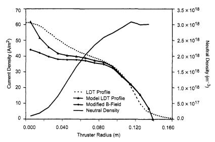
Fig. 4-46. Beam and neutral density profiles at the NSTAR grid [60].
