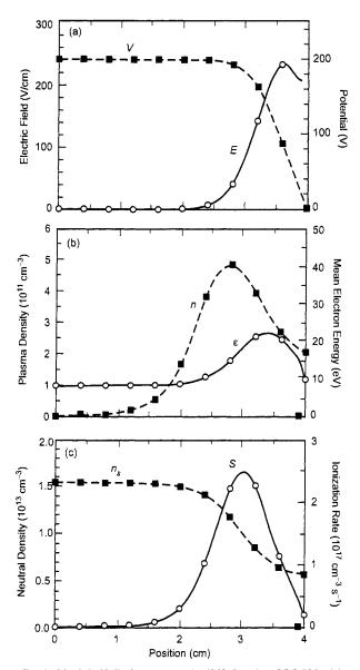
Fig. 7-14. 1-D Hall thruster code [53] for the SPT-100: (a) potential and electric field, (b) plasma density and electron energy, and (c) neutral density and ionization rate (redrawn from [53]).
