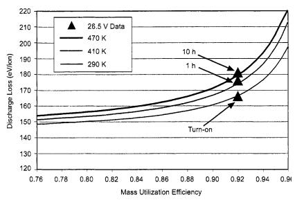
Fig. 4-21. Discharge loss versus mass utilization efficiency from the model for the NEXIS thruster [20] for three neutral gas temperatures,
