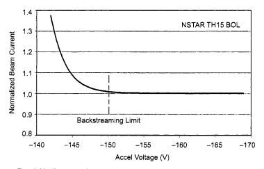
Fig. 5-11. Normalized beam current versus applied accel grid voltage, showing the onset of electron backstreaming as the voltage is decreased.
