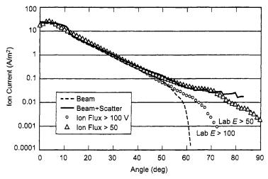
Fig. 8-12. Comparison of high-energy ion current between the calculations and measurements for the BPT-4000 (from [10]).
