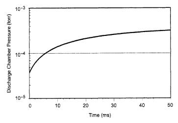
Fig. 4-24. Example of the pressure rise in the NEXIS thruster [20] calculated during a recycle.
