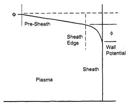
Fig. C-1. Schematic of plasma in contact with the anode wall.
