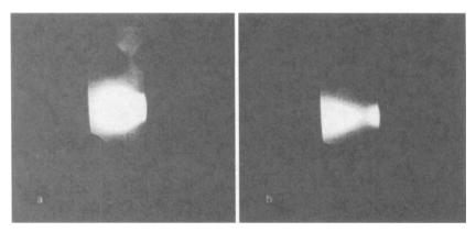
Fig. 6-28. NEXIS cathode plume at 25 A with the plasma ball in (a) at 5.5 sccm and a dark space in (b) at high flow (10 sccm) [1].
