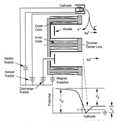
Fig. 7-7. Hall thruster electrical schematic and potential distribution.
