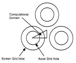
Fig. 5-25. Computational domain of the CEX-3D code (from [17]).
