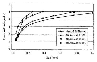
Fig. 5-14. Threshold voltage versus gap for molybdenum after 10 arcs of varying charge transfer (from [36]).
