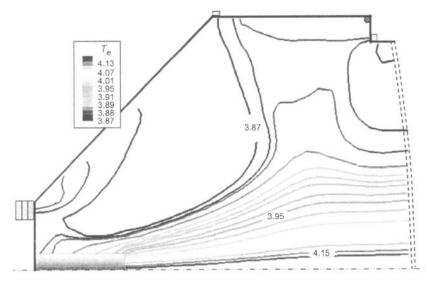
Fig. 4-45. Secondary electron temperatures (eV) for NSTAR thruster at TH15 [60].
