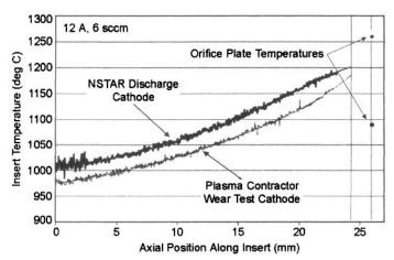
Fig. 6-43. Comparison of the insert temperature profile for the Space Station Contactor cathode and the NSTAR discharge cathode at 12 A (from [33]).
