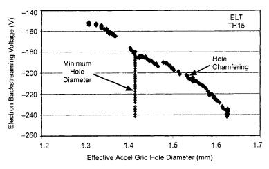
Fig. 5-13. Accel grid voltage at which electron backstreaming occurs in the NSTAR thruster at TH15 power level versus the effective accel grid aperture diameter.
