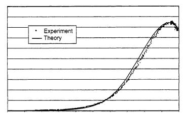
Fig. 6-15. Comparison of the plasma density measured on axis in the NSTAR-sized cathode operating at 12 A and a 4.25-sccm xenon flow with the 2-D code predictions.
