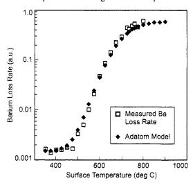
Fig. 6-40. Ba concentration versus cathode surface temperature for -15 V bias. Experimental data are shown by open squares and the model prediction are shown by the diamonds (from [48]).
