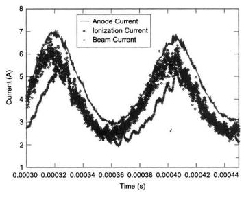
Fig. 7-20. Anode current, ionization, and beam current calculated by HPHall for the SPT-70 Hall thruster (from [30]).
