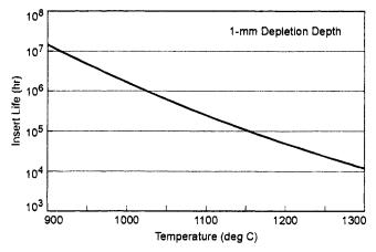
Fig. 6-45. Insert life from barium evaporation calculated for a 1-mm depletion depth versus temperature.
