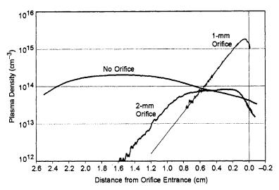
Fig. 6-6. Cathode plasma density profile examples as the orifice diameter is increased for a constant discharge current and flow rate.
