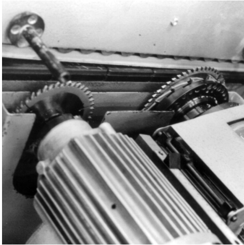
Figure 12 Double-end tenoner machine with horizontal spindles. 8
