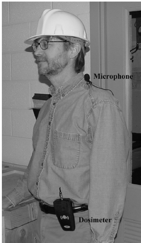
Figure 3 Microphone placement of a noise dosimeter on the shoulder of the wearer.
