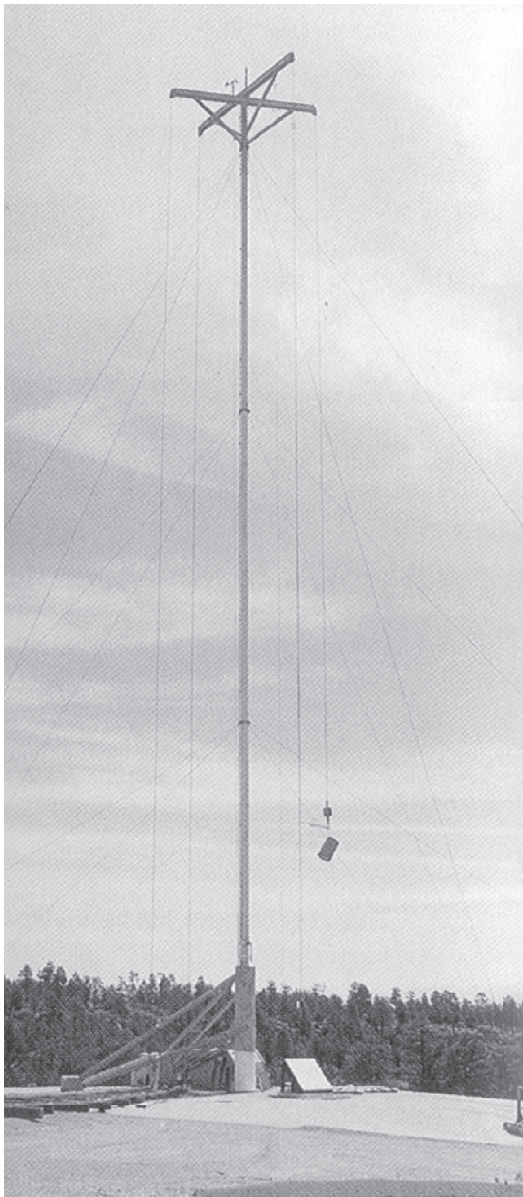
Figure 9 Los Alamos National Laboratory 150-ft drop tower. (From Pusey. 7 )
