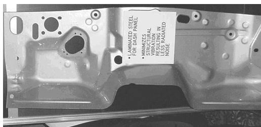
Figure 3 Dashboard panel made of laminated vibration damped steel. 2
