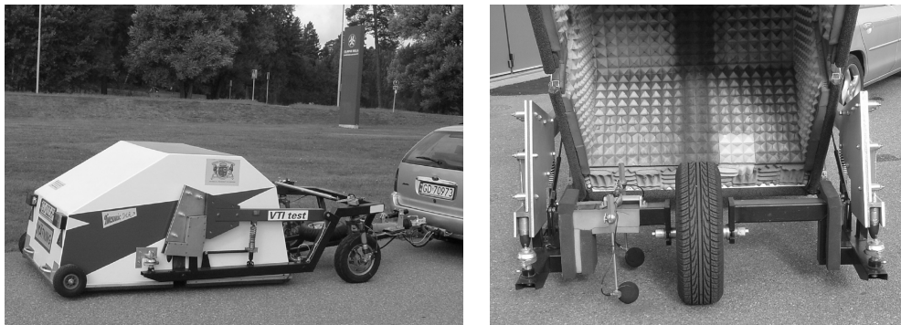
Figure 8 Example of trailer used for measurements with the CPX method. This trailer is from the Technical University of Gdansk in Poland. For characterization of pavements, the method requires the use of two or four reference tires, which are used one at a time. 4
