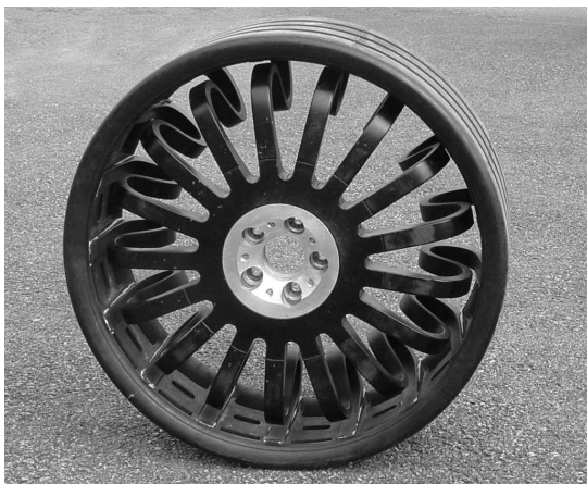
Figure 16 Prototype for a composite wheel. Note the slots in the tread band, which are providing ventilation to the grooves in the tread band. 4
