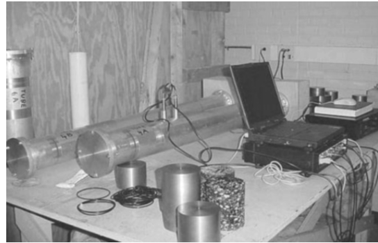
Figure 19 Experimental setup for sound absorption measurements of asphalt road surface samples with impedance tube, microphones A and B, and frequency analyzer. Note the road surface samples and metal spacers. Two 10-cm diameter tubes lie horizontally on the table. One 15-cm diameter tube can be seen standing vertically on the left.
