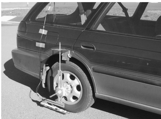
Figure 9 Typical setup for the sound intensity method. 26,27 (Picture used with permission.)
