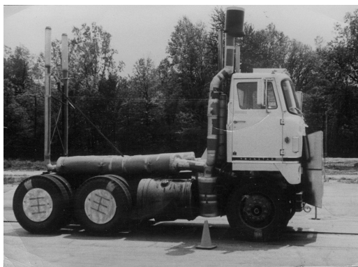
Figure 5 Selective wrapping and oversize muffler used on a diesel engine truck.
