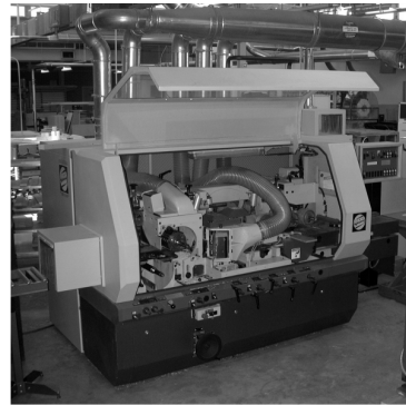
Figure 1 Cutting area of typical industrial moulder machine.
