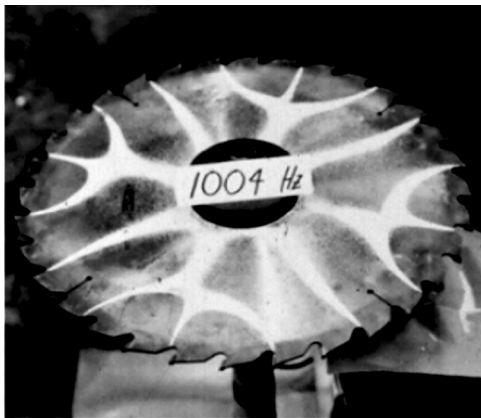
Figure 19 Resonant vibration modal pattern for a circular saw blade (1004 Hz excitation). 10
