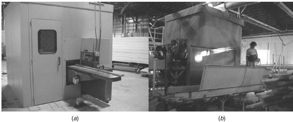
Figure 15 (a) Use of complete panel enclosure for molder noise and (b) use of mass-loaded vinyl "curtains" to control rip saw noise. 71
