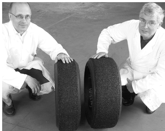
Figure 17 Two prototypes of the porous tread tire, produced by B. Kalman (VTI, Sweden) and A. R. Williams (UK, formerly at Dunlop Tyres).
