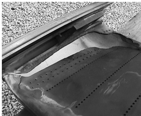
Figure 5.11 Transition failure in GE-F gas turbine due to dynamic stability issues (Tratham, 2001).
