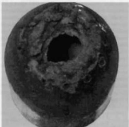
**FIGURE 17.1** Corroded gas tip.
