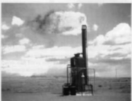
**FIGURE 20.43** Cyclone separator. (Note the frost indicating the flow path of the low-temperature liquid as it is removed.)
