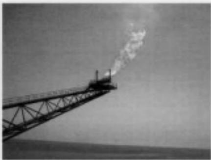
**FIGURE 20.36** Poseidon flare: water-assisted Hydra.
