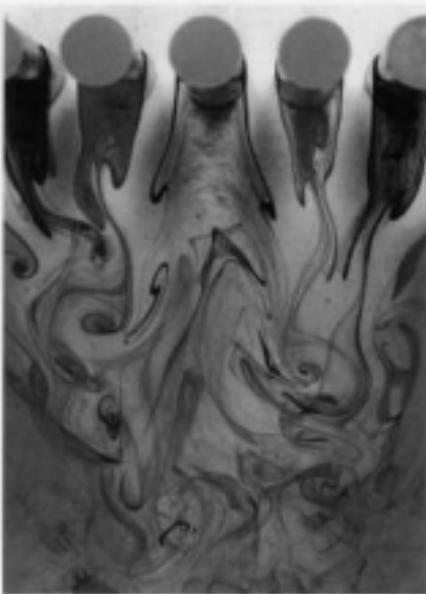
**FIGURE 4.22** Wake area showing mixing vortices. (From Visualization Society of Japan, *The Fantasy of Flow*, IOS Press, Amsterdam, 1993, 3.)
