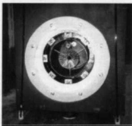
FIGURE 11.7 Typical throat of a raw gas burner.
