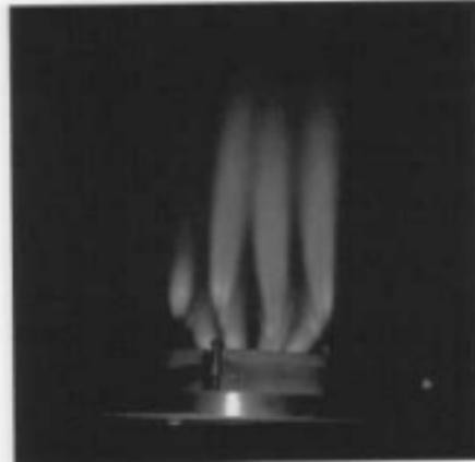
FIGURE 5.14 100% C<sub>3</sub>H<sub>8</sub> flame.
