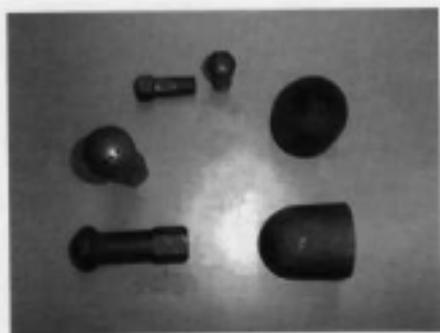
**FIGURE 15.23** Typical fuel gas tips.
