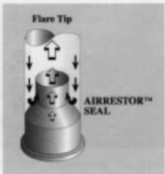
**FIGURE 20.47** Arrestor velocity-type purge reduction seal.
