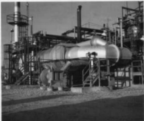
**FIGURE 8.11** Picture of a thermal oxidizer.
