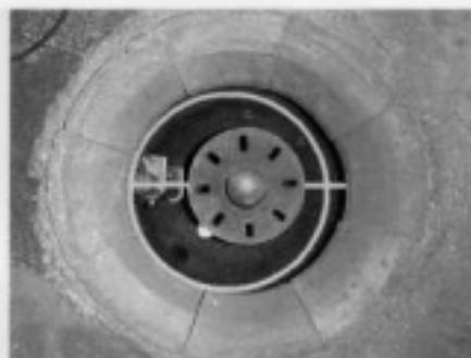
**FIGURE 15.17** VYD burner gas tip in a diffuser with a pilot.
