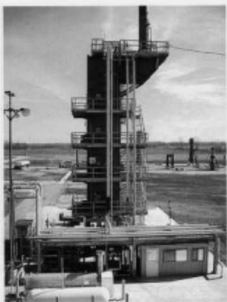
**FIGURE 14.2** Test furnace for simulation of ethylene furnaces.
