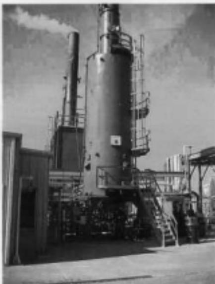
**FIGURE 14.4** Test furnace for simulation of up-fired tests.
