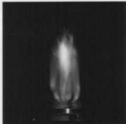
FIGURE 5.18 Simulated reforming gas flame.
