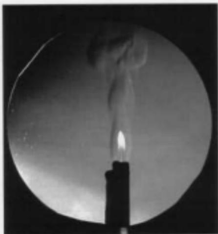
**FIGURE 7.16** Shadow photograph of a burning butane lighter.
