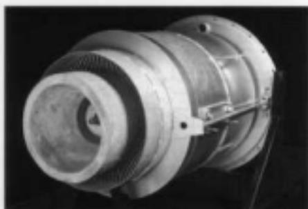
**FIGURE 19.43** An ultra-low emissions burner.
