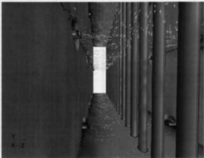
**FIGURE 9.6** Rendered view inside an ethylene pyrolysis furnace showing flow patterns near the premixed radiant wall burners. (Courtesy of John Zink Co.)
