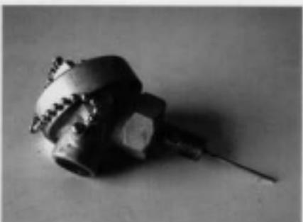
**FIGURE 12.15** Thermocouple.
