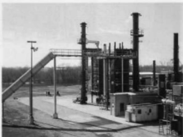
**FIGURE 14.3** Test furnace for simulation of down-fired tests.
