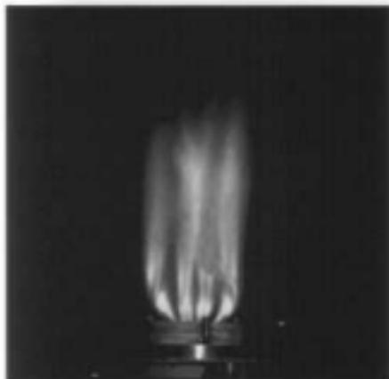
FIGURE 5.15 Simulated cracked gas flame.
