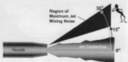
**FIGURE 7.20** Region of maximum jet mixing noise.
