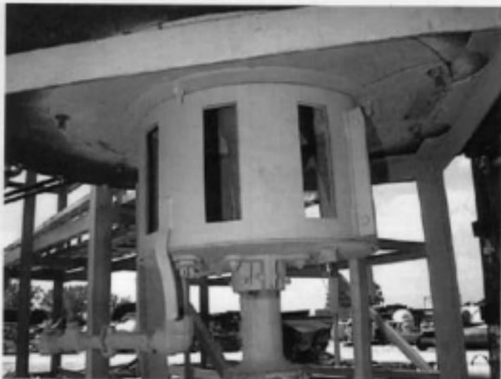
**FIGURE 15.19** Example air register.
