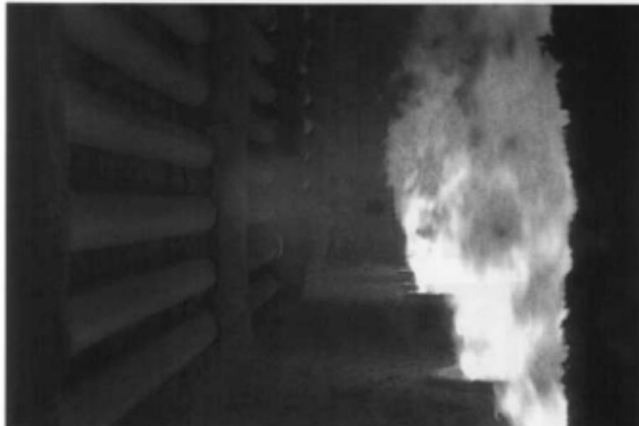
FIGURE 1.21 Crude unit burners.
