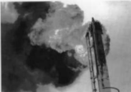
FIGURE 20.21 Typical non-assisted flare.
