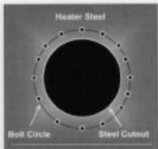
**FIGURE 15.1** Heater cutout and burner bolt circle on a new heater.
