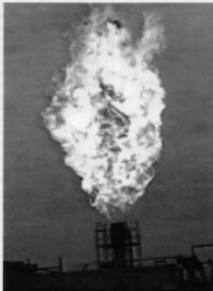
FIGURE 8.28 Annular air-assisted flare; 190,000 lb/hr propane.
