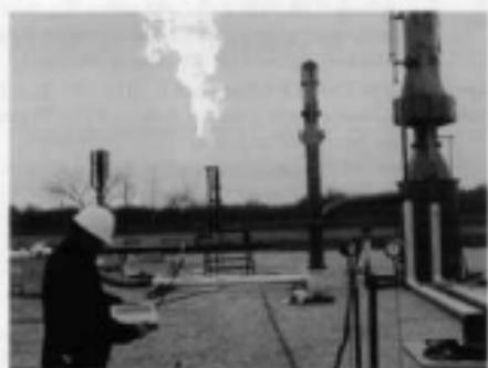
**FIGURE 7.15** Engineer measuring flare noise level.
