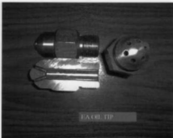
**FIGURE 11.13** Internal mix twin fluid atomizer.
