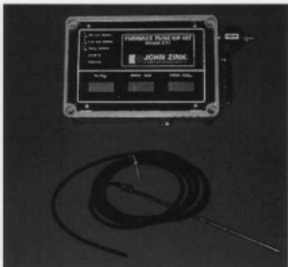
FIGURE 16.5 Oxygen analyzer.
