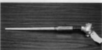
**FIGURE 12.16** Thermowell and thermocouple.
