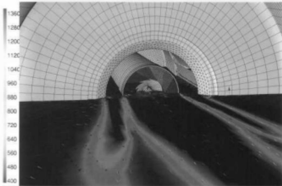
FIGURE 9.18 Mid-plane of geometry colored by temperature (°C). This view shows the burner quard and the mixing regions of acid gas and air.
