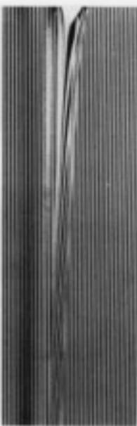
**FIGURE 4.18** Water exiting a faucet at low velocity. (From Visualization Society of Japan, *The Fantasy of Flow*, IOS Press, Amsterdam, 1993, 96.)
